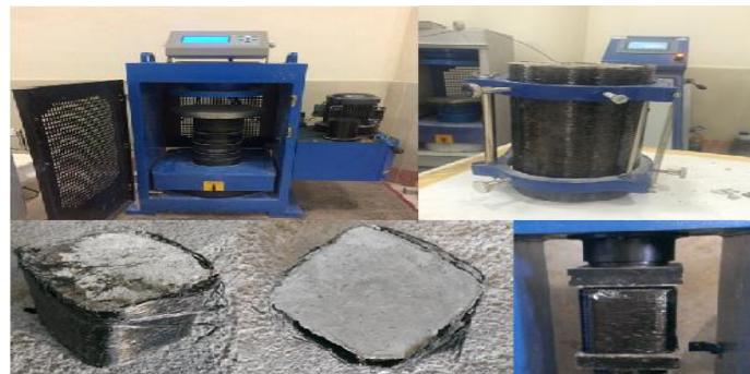
Figure 3. Samples manufactured for compressive strength and stress-strain tests
