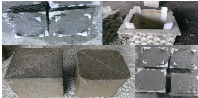
Figure 2. How to make rounded the cubic samples
