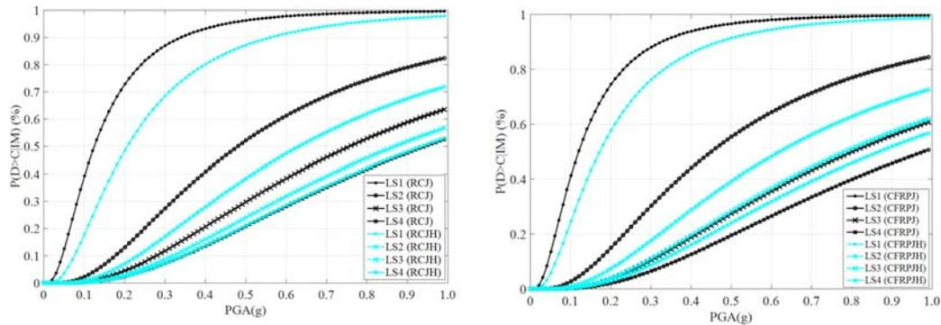
Figure 10. Fragility curves of the bridge piers retrofitted with RC (left) and CFRP (right) jackets considering component-based limit state thresholds according to the proposed methodology (RCJ, CFRP) and HAZUS recommendations (RCJH, CFRPH)
