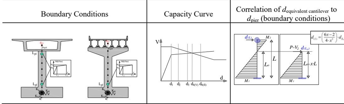
Figure 2. Calculation of limit state thresholds in displacement terms (global engineering demand parameter)
