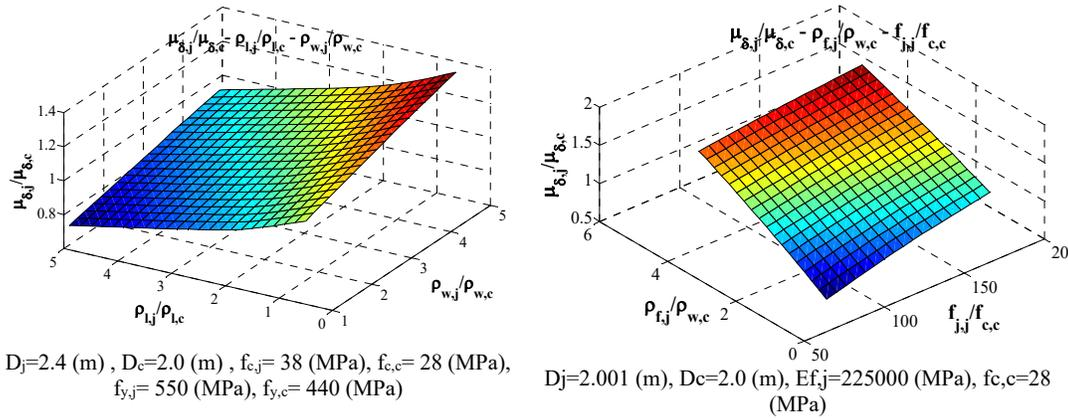
Figure 3. Effect of various parameters on displacement ductility of as-built and retrofitted piers (retrofit with R/C(left) and CFRP(right) jacketing)
