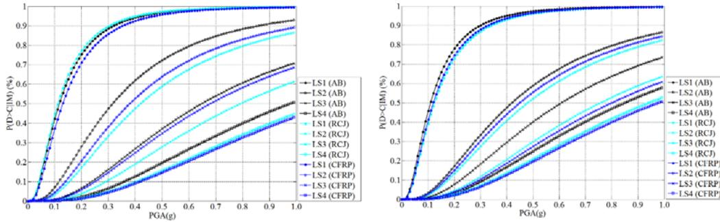
Figure 7. Fragility curves of the as-built (AB) and retrofitted with RC (RCJ) and FRP (CFRP) jacket bridge (longitudinal (left) and transverse (right) direction)
