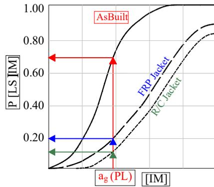
Figure 9. Optimum selection of retrofit measure according to the selected performance level
