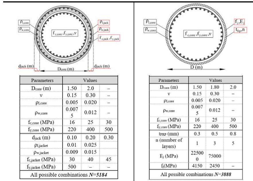
Figure 1. Parameters considered for cylindrical piers retrofitted with R/C and FRP jackets
