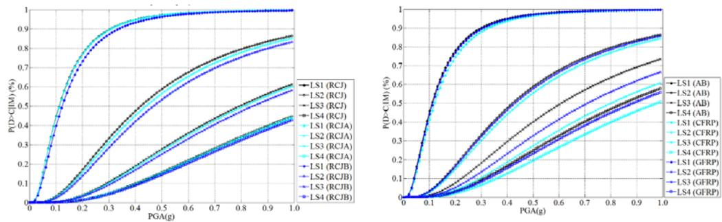
Figure 8. Fragility curves of the longitudinal direction retrofitted with RC jackets (RCJ, RCJA, RCJB) (left) and the transverse direction retrofitted with FRP jackets (CFRP and GFRP)
