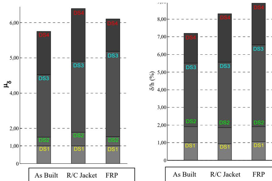
Figure 4. Limit state thresholds of retrofitted bridge piers (R/C and FRP jackets) in terms of displacement ductility ( $\mu_\delta$ ) and drift ( $d/h$  %)
