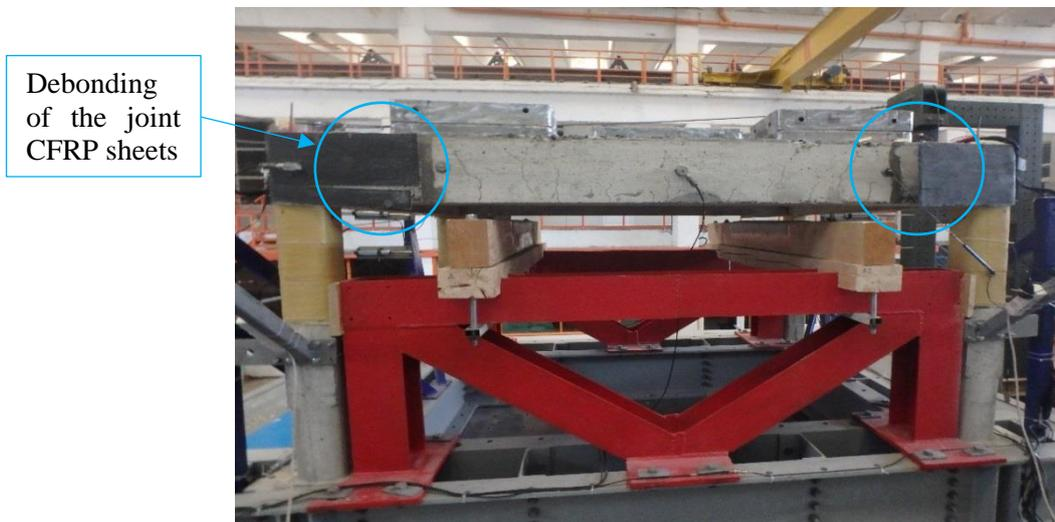
Figure 6: CRuRC frame after testing, showing the de-bonding of CFRP sheets and beam flexural cracks (X direction)
