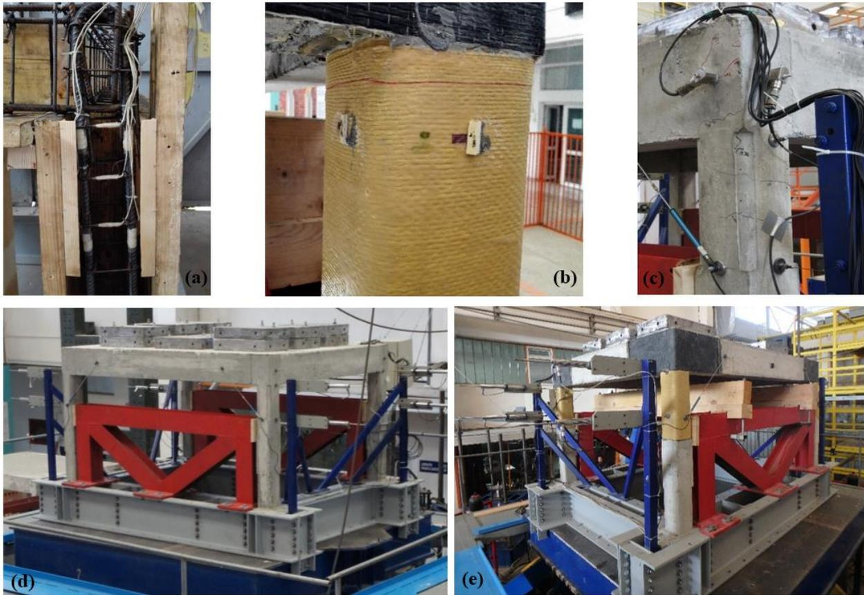
Figure 3: (a) Reinforcement cage in place with strain gauges connected, (b) Strain gauges on the AFRP, (c) Accelerometers and inclined LVDT, (d) RC frame prior to testing, and (e) RuC frame prior to testing
