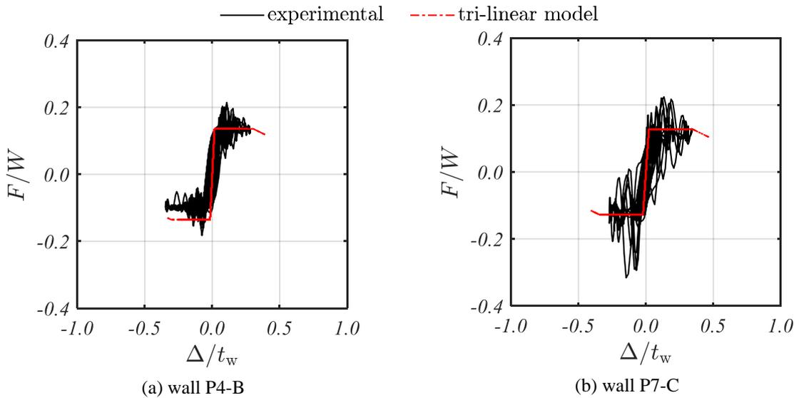
Figure 4 Shake table tests carried out at the University of Auckland (Giarretton et al., 2016): simulation by means of the proposed tri-linear model. Force-displacement response.
