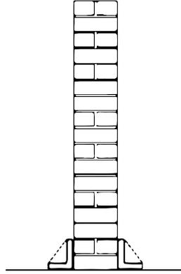
Figure 3 Cross-section of the walls tested on the shake table by (Giarretton et al., 2016).
