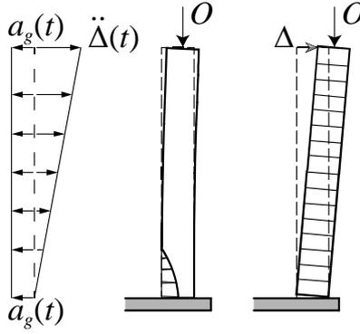
Figure 2 URM cantilever or parapet walls, from (Godio and Beyer, 2018).
