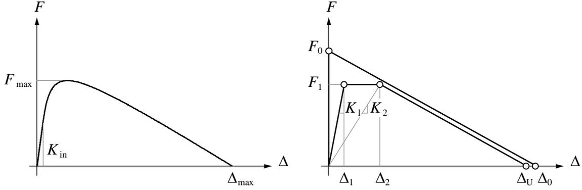
Figure 1 Left: typical pushover curve of vertically-spanning URM walls. Right: bi- and tri-linear idealisations. From (Godio and Beyer, 2018).
