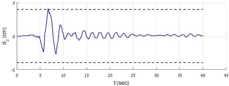
Figure 5 Response of the second inter-story drift (i.e.  $d_2(t)$ ) of the structure with the optimized distribution of dampers. The dashed line represents the maximum allowable value of the drift at location 2 (i.e. 3.96 cm)
