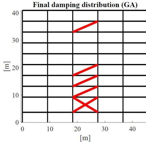
Figure 6 Final damping distribution having 9 potential locations for dampers. Locations 1, 2, 3, 4, and 8 are actually occupied by dampers in the final solution. Only one size-group of dampers is actually present in the solution:  $\bar{c}_2 = 497.49$  [kN(s/mm) <sup>$\alpha$</sup> ]
