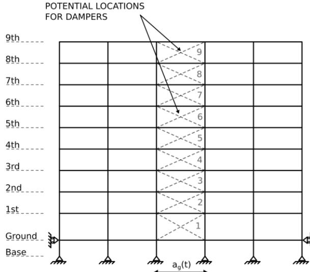
Figure 4 Potential locations for dampers in the nine-story moment resisting frame.
