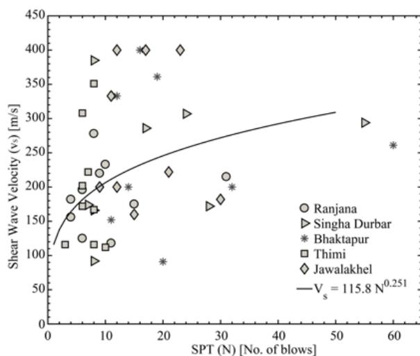
Figure 3. Comparison of measured shear wave velocity ( $V_S$ ) with uncorrected SPT-N values at five sites across Kathmandu. The trendline shown is from the regression study performed by Gautam (2017) on a different data-set and is described by the equation  $V_S = 115.8 N^{0.251}$  ( $R^2 = 0.623$ ).
