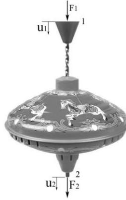
Figure 1. A physical realization of the inerter which is the mechanical analogue of the capacitor in a force-current/velocity-voltage analogy.
