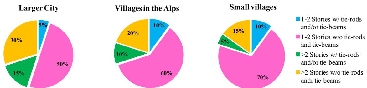
Figure 4. Building stock subdivision into structural typologies, based on the environmental context.
