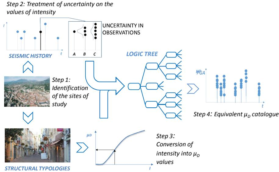
Figure 1. Sketch of the proposed methodology to convert macroseismic intensities into mean damage values (adapted from Rota and Rosti 2017).
