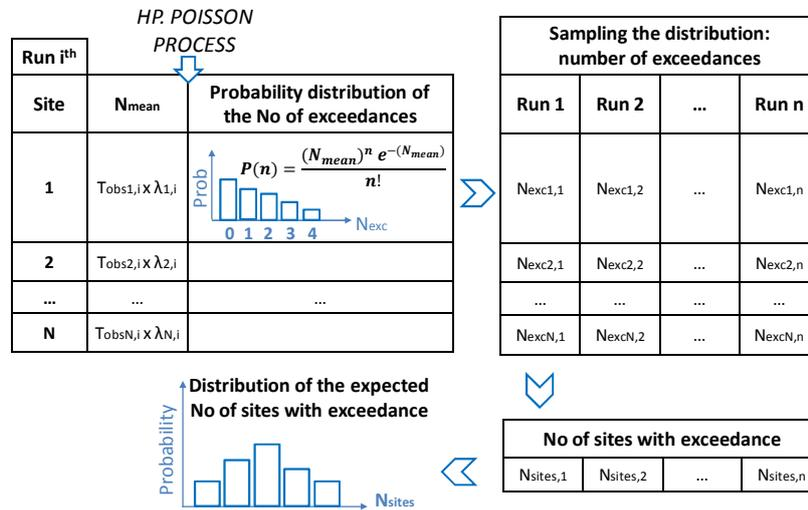
Figure 3. Sketch of the procedure to generate number of exceedances compatible with the PSH model. Calculation of the number of sites with exceedance and of its distribution for a given mean damage threshold (adapted from Rota and Rosti 2017).
