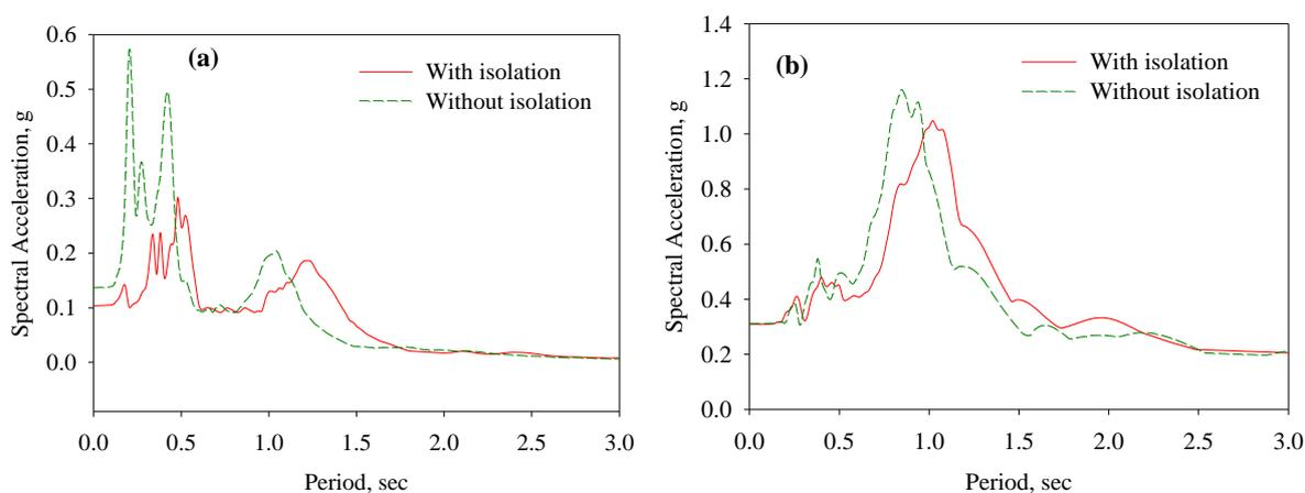
Figure 7. Response spectra at the footing level for (a) Myanmar and (b) Nepal earthquakes
