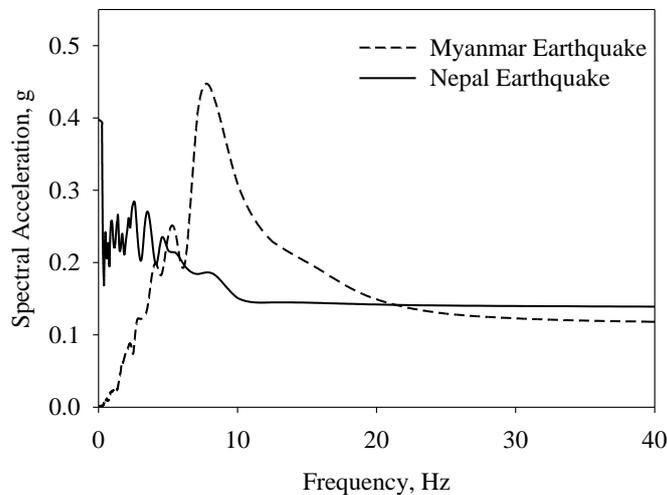
Figure 3. Response spectra of input motions
