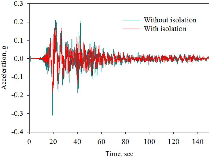
Figure 6. Acceleration-time history at the footing level for Nepal earthquake
