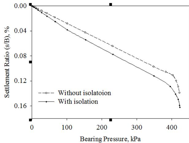
Figure 4. Bearing pressure- settlement response under static loading
