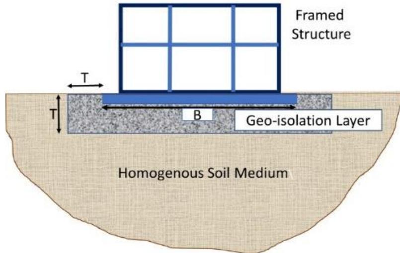
Figure 1. SRM- isolation system used for earthquake protection of building
