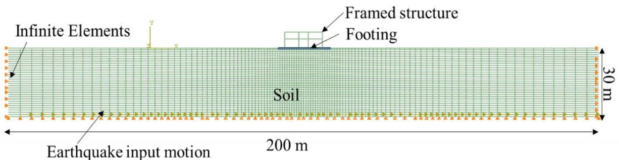
Figure 2. Finite element model of geo isolated structure
