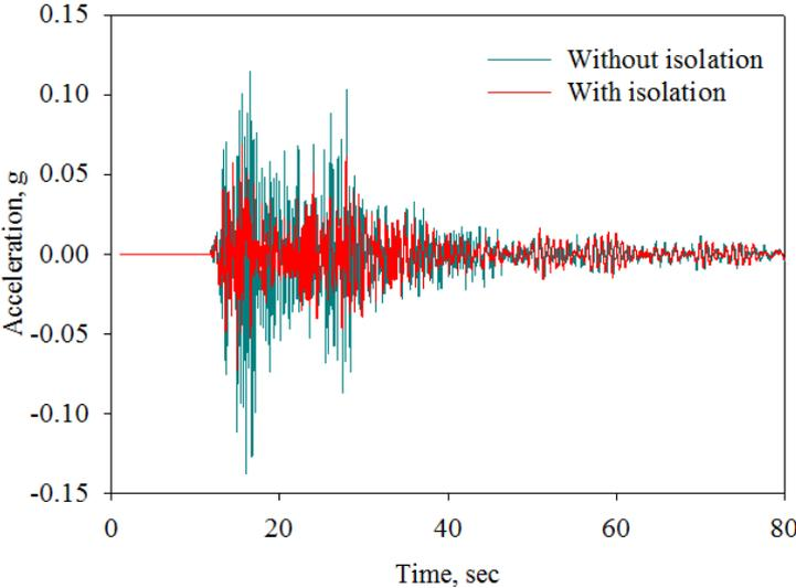
Figure 5. Acceleration-time history at the footing level for Myanmar earthquake
