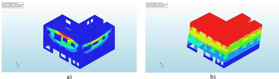
Figure 12. Analysis results: a) the first eigen mode of the building in a damaged state ( $T_1 = 1.25$  s), b) the first eigen mode with R.C. floors added ( $T_1 = 0.35$  s)
