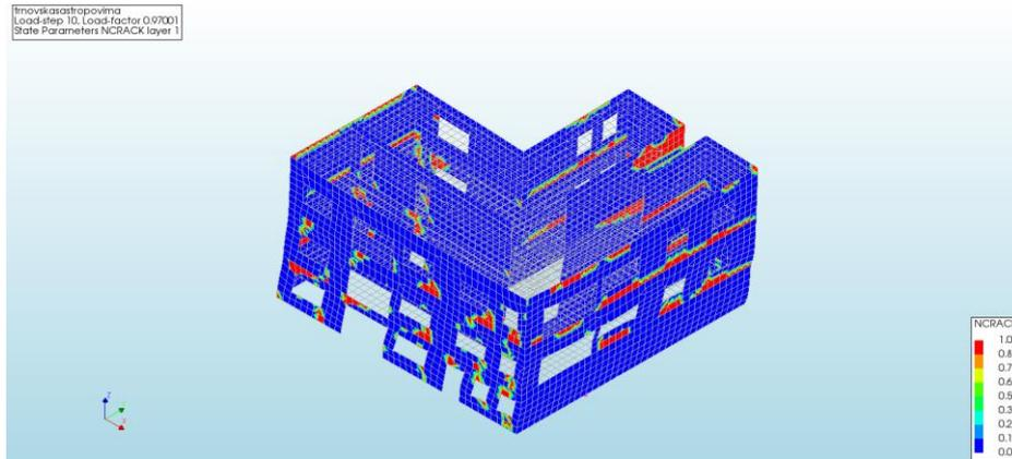
Figure 13. Analysis results – cracking in the damaged state
