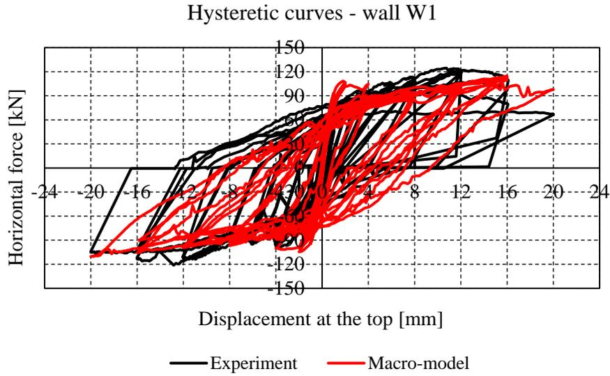
Figure 5. Comparison of hysteretic curves of the macro-model and the experiment for W1
