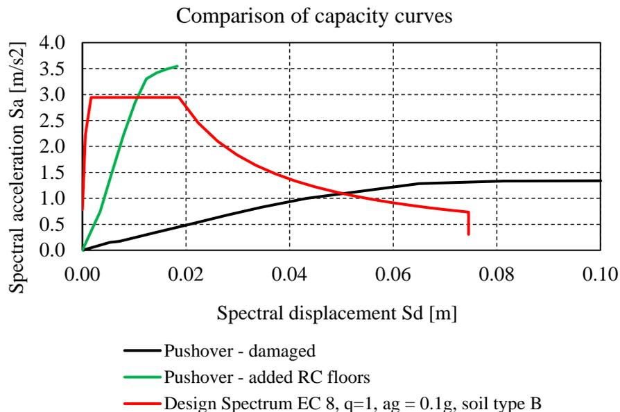
Figure 14. Comparison of capacity curves of existing damaged building and the building with R.C. floors
