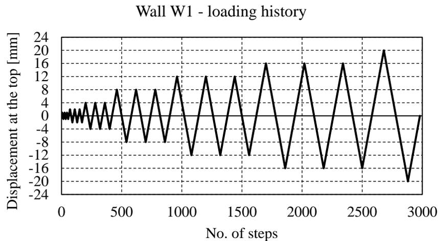
Figure 4. Loading program for wall W1
