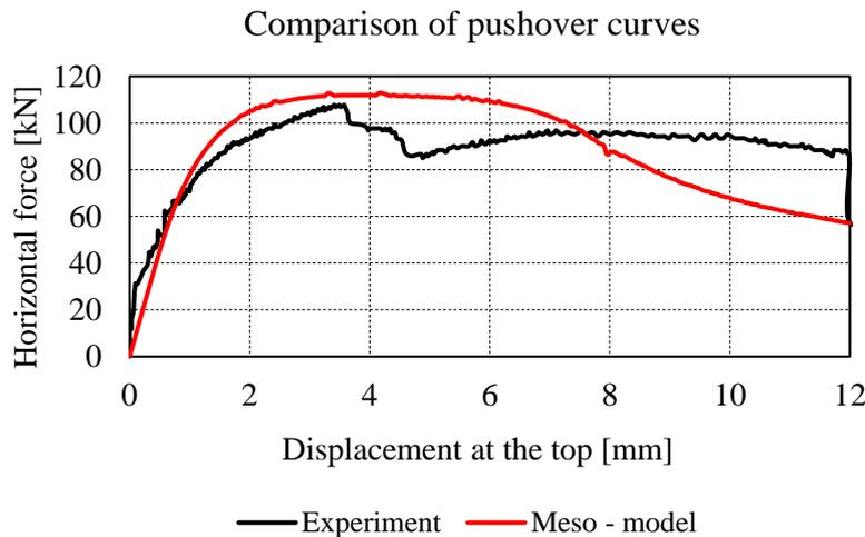
Figure 10. Comparison of pushover curves obtained experimentally and numerically
