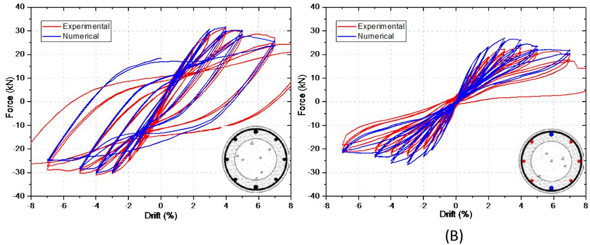
Figure 6. Load-deformation diagrams: (A) HFA-Tube, (B) HFA-Tube-SEA
