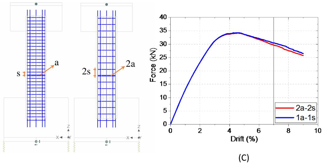
Figure 8: Effect of spacing of transverse reinforcement in HFA-Tube: (A) actual spacing (1a-1s), (B) doubled spacing with doubled reinforcement area (2a-2s), (C) load-deformation diagrams.
