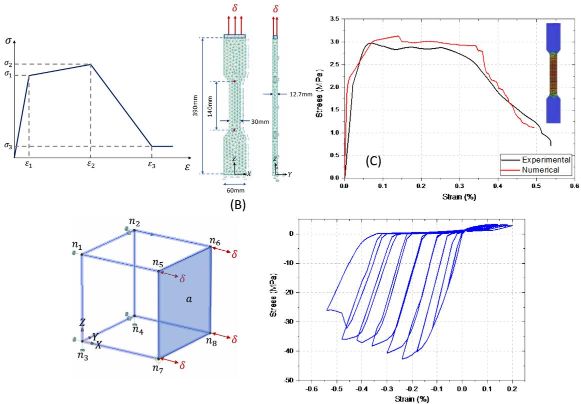
Figure 2. ECC modeling approach: (A) schematic stress-strain behavior of smeared reinforcement, (B) modeled dog-bone specimen, (C) stress-strain diagram for modeled dog-bone specimen, (D) single brick element, (E) stress-strain response from brick elements under to cyclic loads
