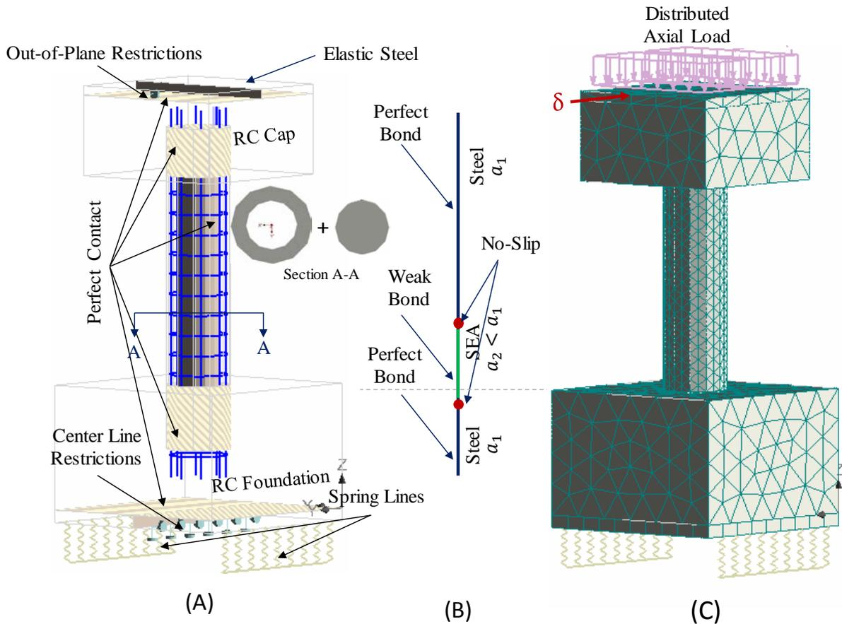
Figure 5. Numerical models: (A) geometry, reinforcement, and boundary condition, (B) modeling of Cu-Al-Mn SEA bars and steel rebar, (C) mesh and loading
