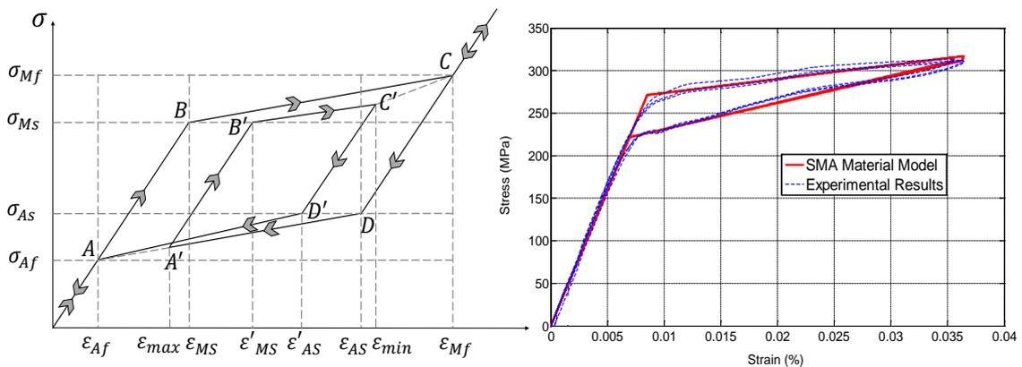
Figure 3. Constitutive model for SEA: (A) theoretical behavior, (B) calibrating the model with experimental data
