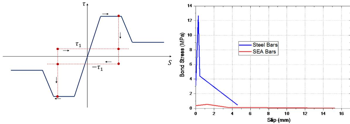
Figure 4. “Memory Bond” material: (A) general cyclic behavior, (B) bond-slip diagrams for reinforcing steel and Cu-Al-Mn SEA bars
