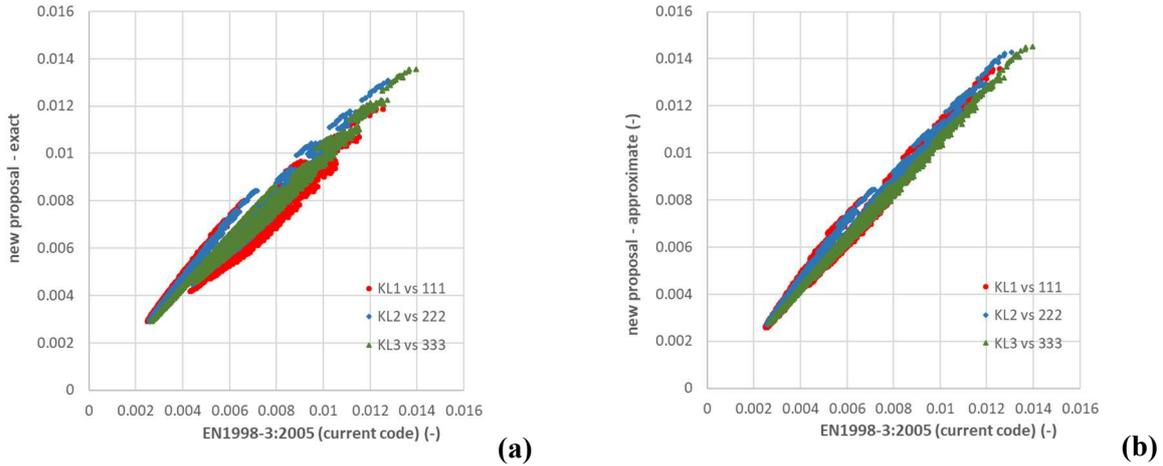
Figure 4. Ultimate chord rotation of RC members, diagonal cases,  $i=j=k$ : (a) New capacity with “exact” case-dependent  $\gamma_{Rd}$ ,  $R_{ijk}$ , vs former capacity  $R_{KLi}$ ; (b) New approximate capacity (average  $\gamma_{Rd}$ ) vs former capacity.
