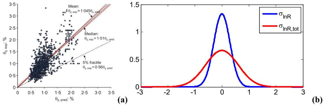
Figure 1. Capacity models: (a) experimental vs predicted values of chord rotation at yield for a RC member, according to the model in (Biskinis and Fardis, 2010); (b) increased dispersion of predicted capacity with respect to actual capacity (for an assumedly unbiased model).
