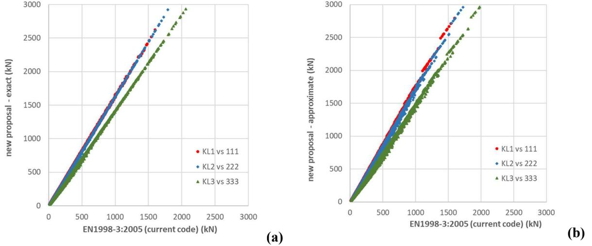
Figure 3. Shear resistance of RC members, diagonal cases,  $i=j=k$ : (a) New capacity with “exact” case-dependent  $\gamma_{Rd}$ ,  $R_{ijk}$ , vs former capacity  $R_{KLi}$ ; (b) New approximate capacity (average  $\gamma_{Rd}$ ) vs former capacity.
