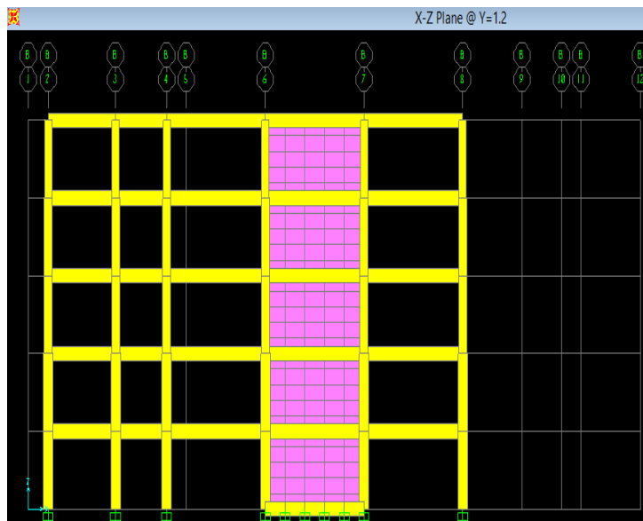
Figure 8. Modeling of shear wall in direction XZ at Y=1.2 m
