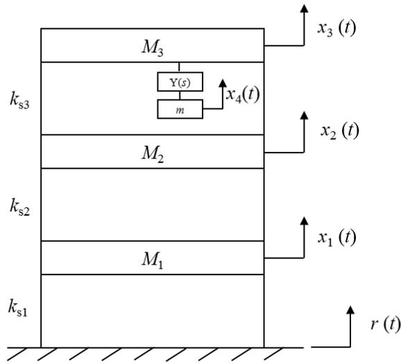
Figure 3. Three-storey building model with the vibration absorber mounted on the top
