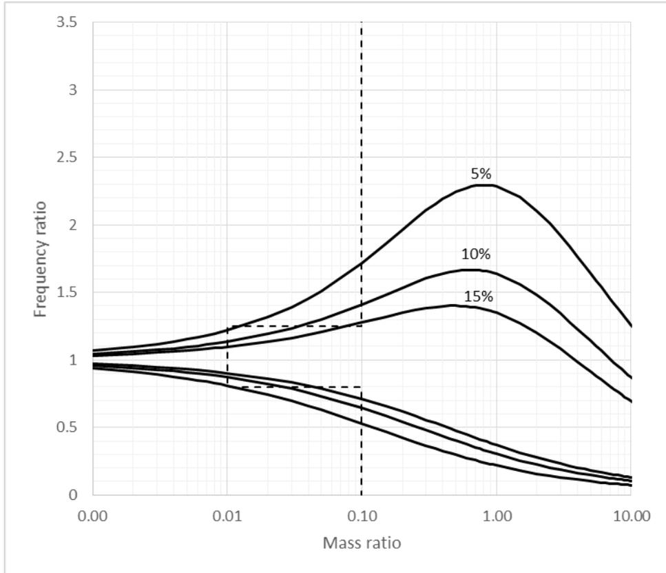
Figure 6. Curves for error of 5%, 10% and 15% in response values if the system is uncoupled
