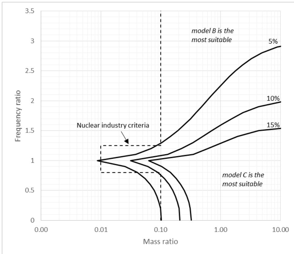
Figure 4. Curves for error of 5%, 10% and 15% in the natural frequency if kinematic interaction is neglected
