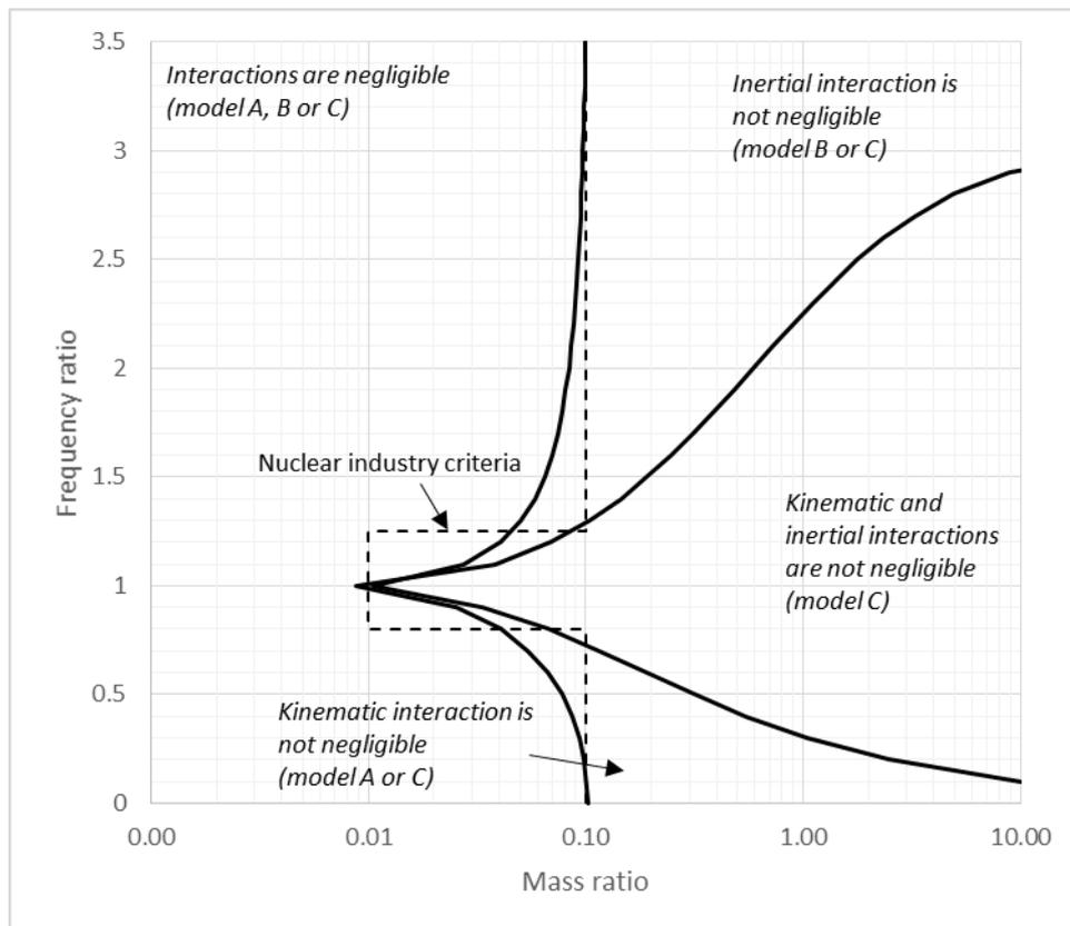
Figure 5. Decoupling criteria for frequency changes in the space of frequency and mass ratios
