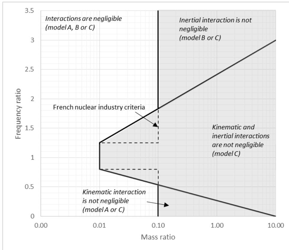
Figure 8. New dynamic decoupling criteria for use in seismic analysis.
