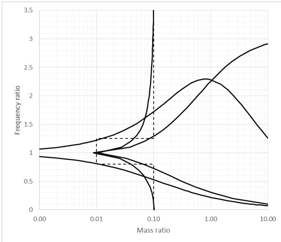
Figure 7. Decoupling criteria for a 5% change in response and frequencies of the primary system
