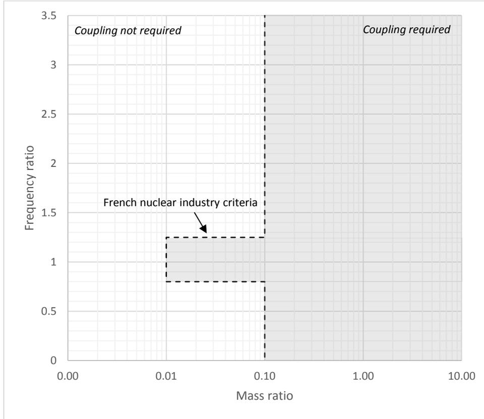
Figure 1. Decoupling criteria applied in the nuclear industry.
