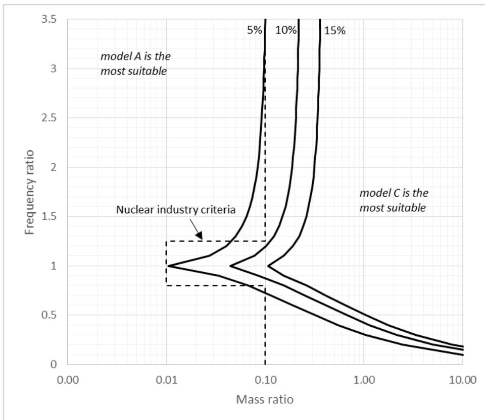
Figure 3. Curves for error of 5%, 10% and 15% in the natural frequency if the system is uncoupled.
