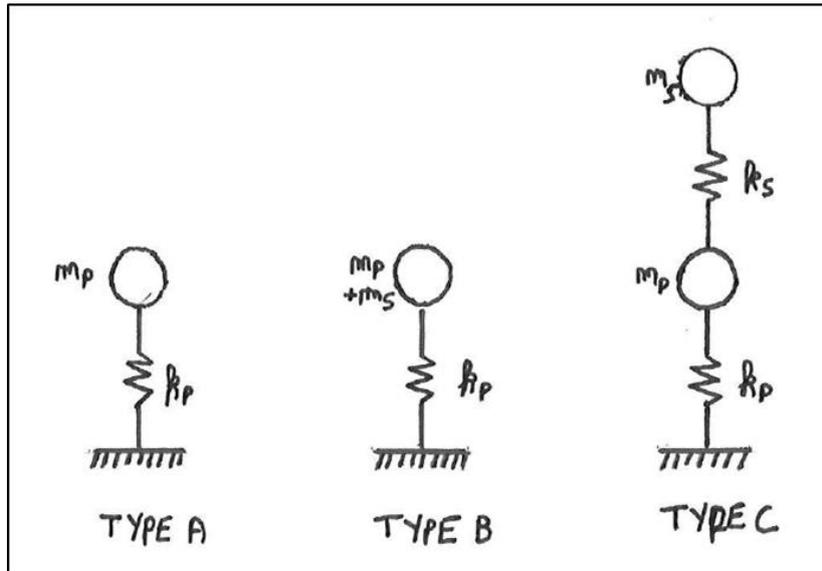
Figure 2. Models for analyzing decoupling criteria.
