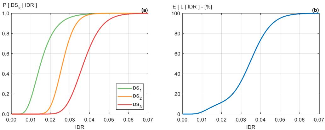
Figure 8. (a) Fragility curves; and (b) Expected loss ratio as a function of IDR, for interior structural walls (component number B1071.021 of ATC-58 project (Hamburger et al. 2004)).
