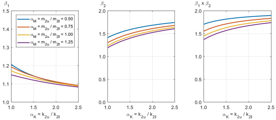
Figure 4. Variation of  $\beta_1$ ,  $\beta_2$ , and  $\beta_1 \times \beta_2$  in 2-story models, as a function of their mass and stiffness distribution coefficients, using the first modal shape and constant story heights.
