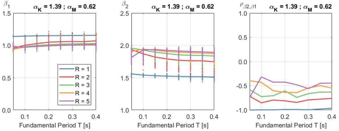
Figure 5. Variation of  $\beta_1$  and  $\beta_2$  in 2-story models as a function of their fundamental period of vibration and  $R$ , using  $\alpha_K = 1.39$ ,  $\alpha_M = 0.62$ , and constant story heights. Results of individual records are presented as points, and their geometric means as solid lines.
