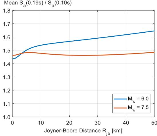
Figure 2. Median ratio between spectral ordinates at 0.19s and 0.10s as a function of  $M_w$  and  $R_{jb}$ , according to the GMPM developed by Boore et al. (2014), with  $V_{s30} = 250$  m/s.
