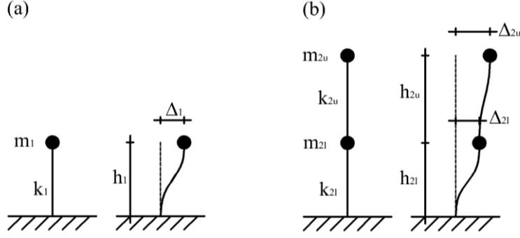
Figure 1. Simplified lumped mass models. (a) 1-story model; (b) 2-story model.
