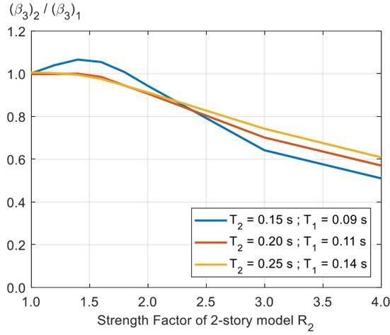
Figure 7. Variation of the median ratio  $(\beta_3)_2 / (\beta_3)_1$  as a function of the strength factor and fundamental period of the 2-story model, with a constant ratio  $T_2 / T_1 = 1.76$ .
