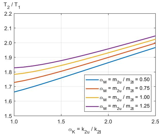
Figure 3. Variation of the period ratio between 2- and 1-story houses as a function of mass and stiffness distribution coefficients.
