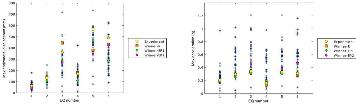
Figure 1 - Plots of predicted maximum displacement (left) and maximum acceleration (right) at the top of the column for each earthquake in the PEER contest (Terzic et al. 2015).
