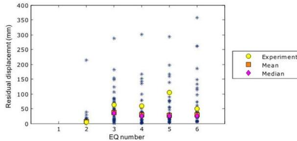
Figure 2 - Plot of predicted residual displacement at the top of the column after each earthquake in the PEER contest (Terzic et al. 2015).
