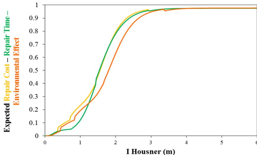
Figure 4. Economic-Resilient-Environmental seismic scenarios for 4 story BareFrame OldCode type.
