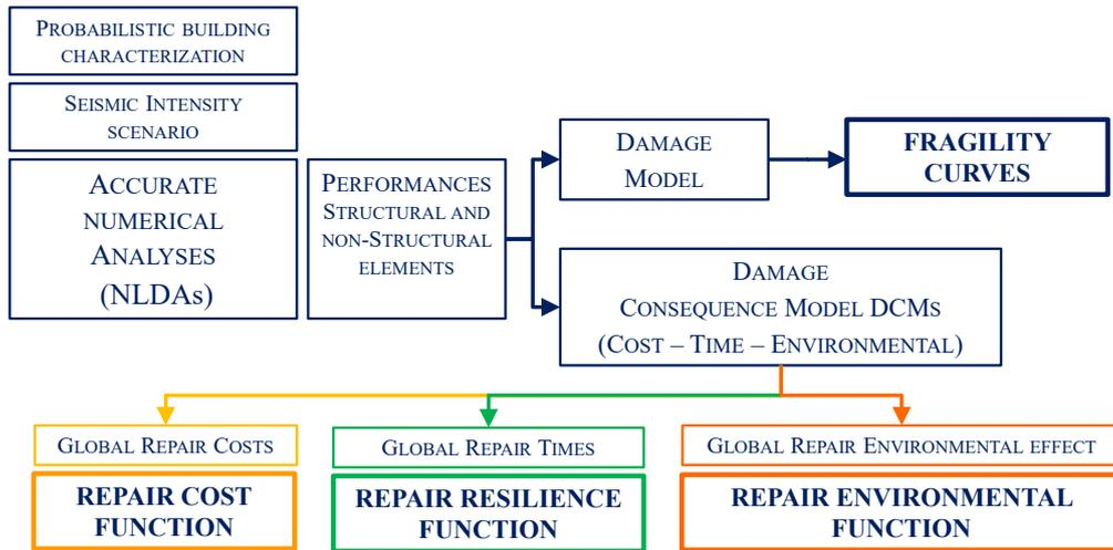
Figure 1. Flowchart of the proposed procedure in defining the main items of a Seismic scenario.
