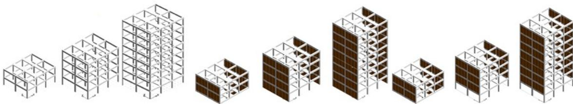
Figure 2. Geometric characteristics of the RC-MRF building types analysed - Storey number (2,4,8) and infill panels distribution and effectiveness (Bareframe BF, InfillFrame IF, PilotisFrame PF).
