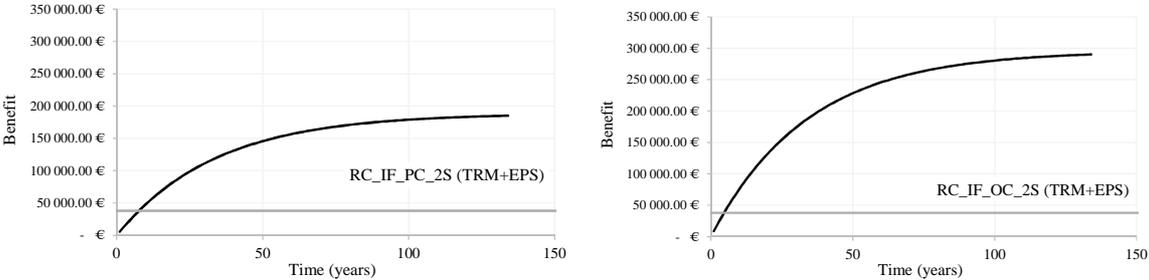
Figure 8: Intersection between the NPV-Time curves and the intervention cost for two Infilled frame typologies (Pre code – Old Code) retrofitted by mean the TRM + EPS integrated system (for the seismic region 1 and the climatic zone F).
