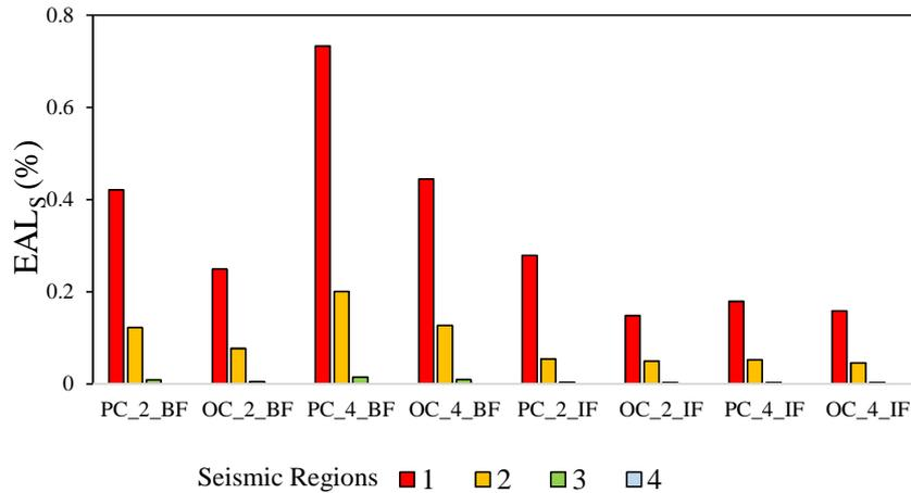
Figure 3: Seismic Expected Annual Losses ( $EAL_S$ ) values for the considered RC-MRF typologies in as-built condition and for the four Italian seismic regions (1-2-3-4)
