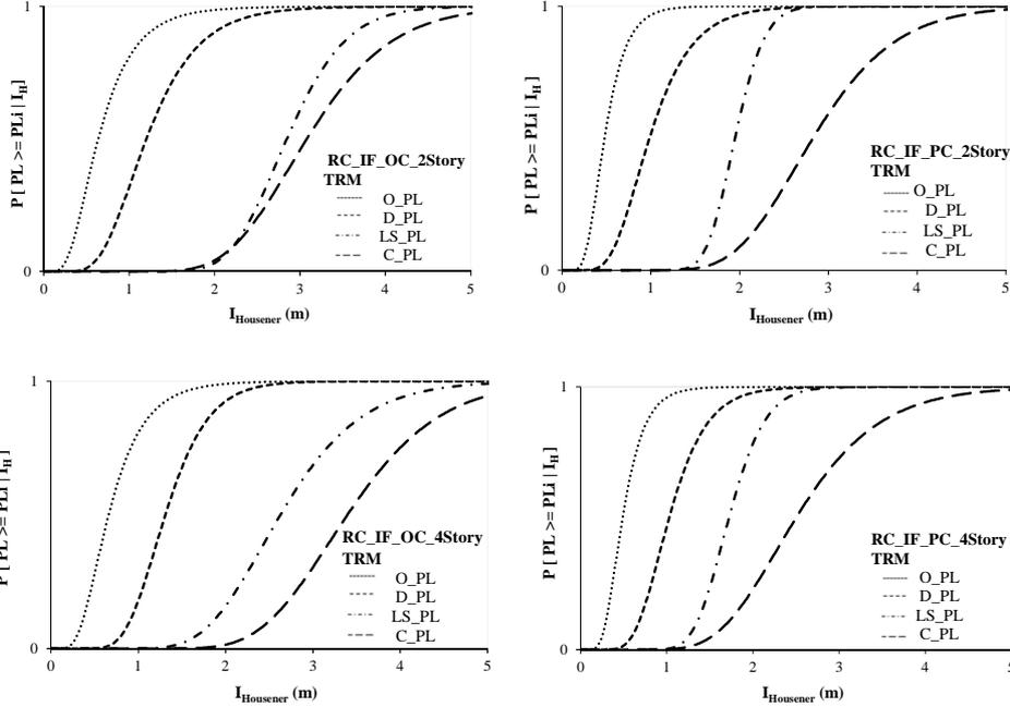
Figure 6: Fragility curves for Infilled frame RC-MRF typologies after the retrofitting with TRM jacketing of infills, defined according to the simplified procedure.
