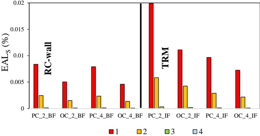
Figure 7:  $EAL_S$  values for the considered RC-MRF typologies in retrofitted condition and for the four Italian seismic regions (1-2-3-4).
