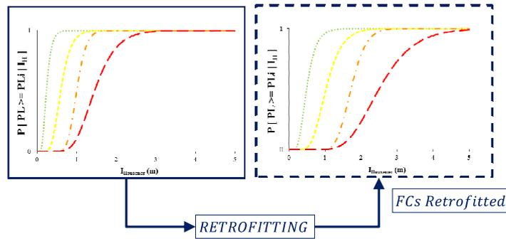
Figure 2: Comparison between the fragility curves in as-built and retrofitted state.
