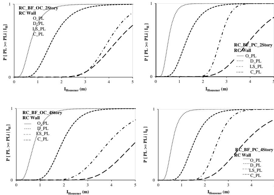
Figure 5: Fragility curves for bare frame RC-MRF typologies after the retrofitting with RC-wall, defined according to the simplified procedure.
