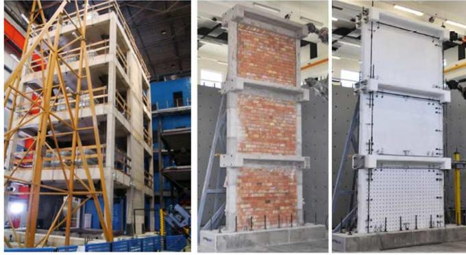
Figure 4: (a) RC-MRF 4 story prototype retrofitting with two infilled RC-wall in transversal direction proved in Elsa lab (Chrysostomou et al. 2013); (b) RC-MRF 3 storey frame of a 2:3 prototype retrofitted with masonry infills TRM Jacketing proved in Patras University Lab (Koutas et al. 2015).
