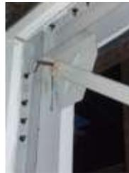
Failure of welded connection between steel frame and brace at drift 1/75.
