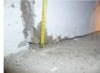
Lifting (10mm) of strengthened masonry wall at drift 1/100
