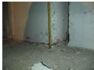
Lifting (25mm) of central wall at drift 1/75
