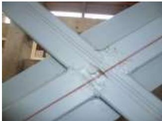
Damage initiation of brace at drift 1/200
