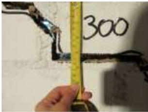
Separation of bricks (10mm) at drift 1/100
