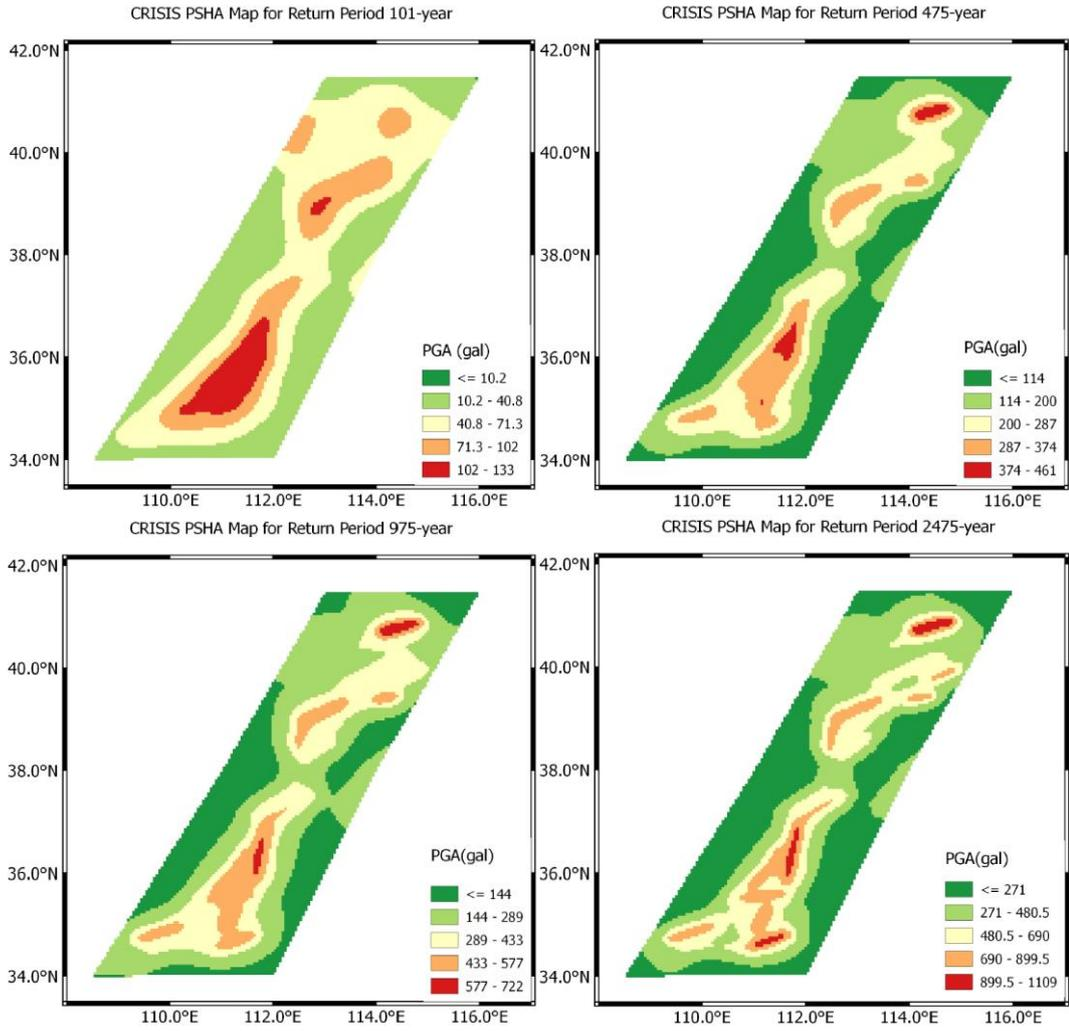
Figure 3: Modelled hazard maps using CRISIS2015 based on PSHA method for return period 101-yr, 475-yr, 975-yr and 2475-yr, respectively (unit: gal, 1g=981gal).
