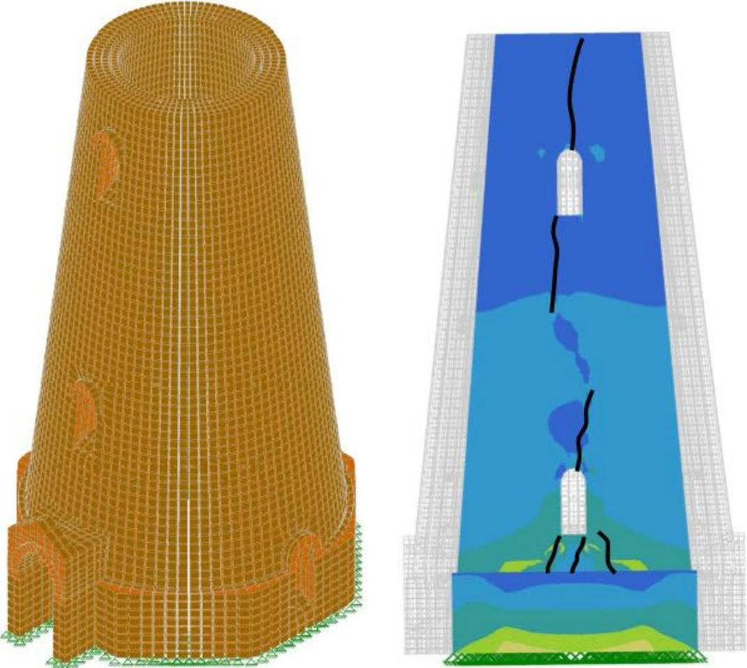
Figure 3. Computational model of tower and crack mapping comparison to stresses (RISA, 2016)
