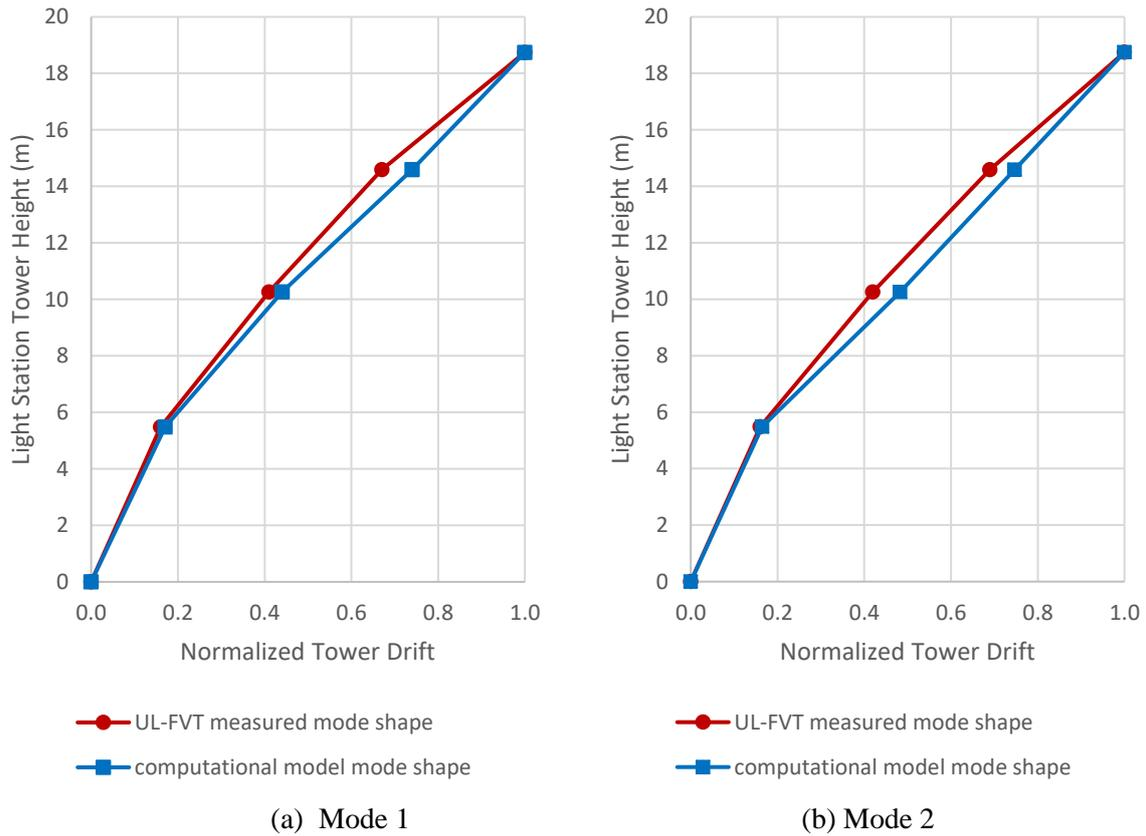
Figure 5. Normalized UL-FVT and computational mode shape comparison
