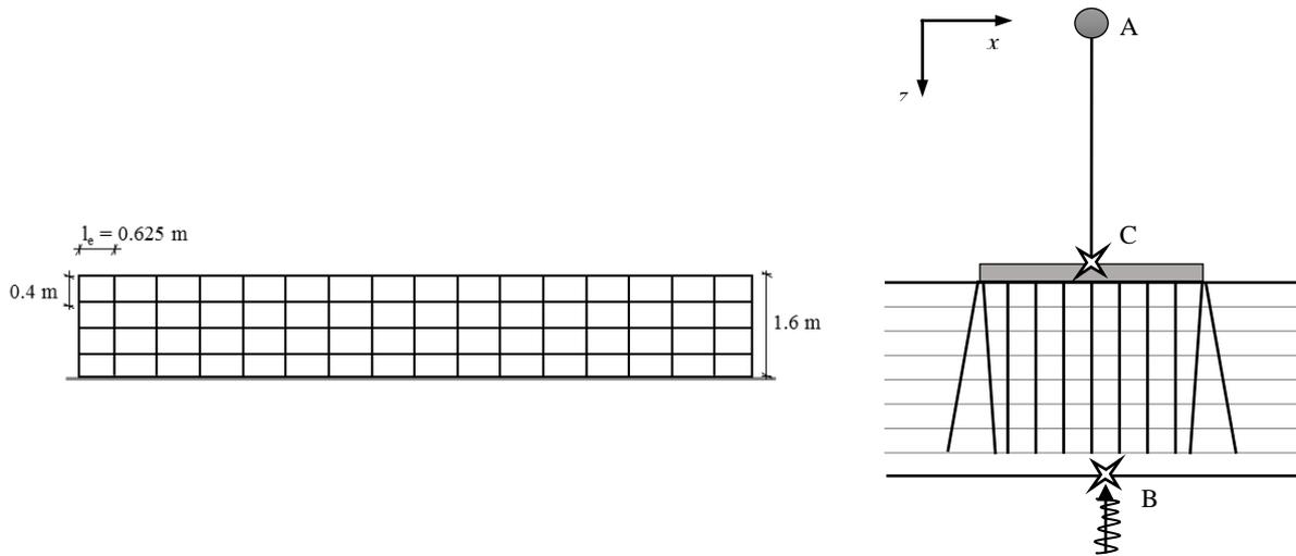
Figure 3. (left) Element size in the foundation mesh. (right) Tower model on a multi pile grid on the layered soil model The investigation point A is located at the tower top mass, point B is placed on the top of the stiff bedrock, point C at the foundation top.
