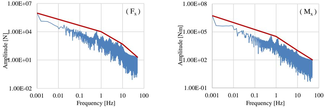
Figure 6. Envelope curve of horizontal wind force and overturning moment acting on the reference turbine.
