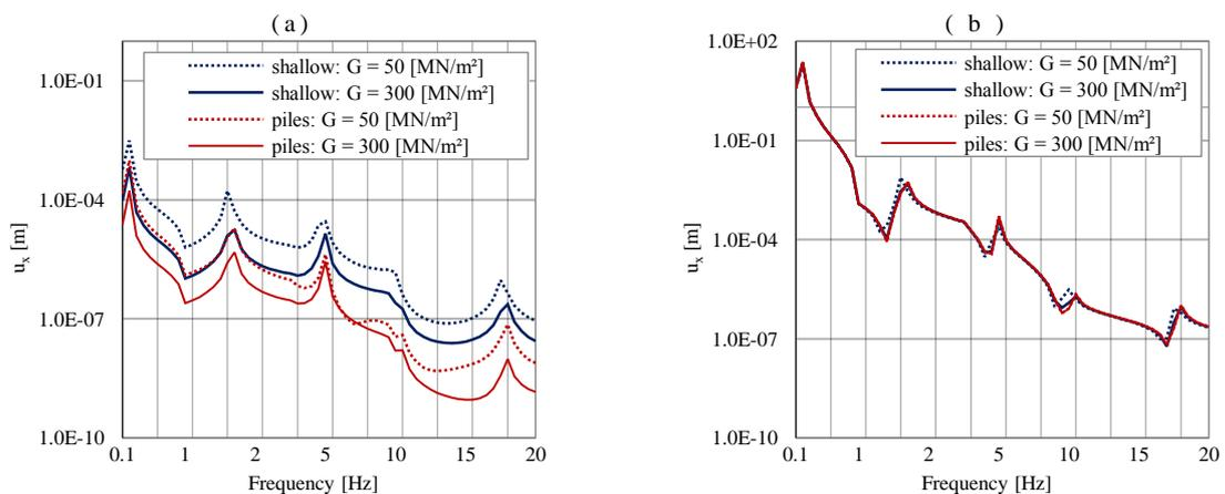
Figure 7. Horizontal displacement at the foundation top edge (left) and at the tower top (right) under a frequency dependent wind load applied at the tower top node.
