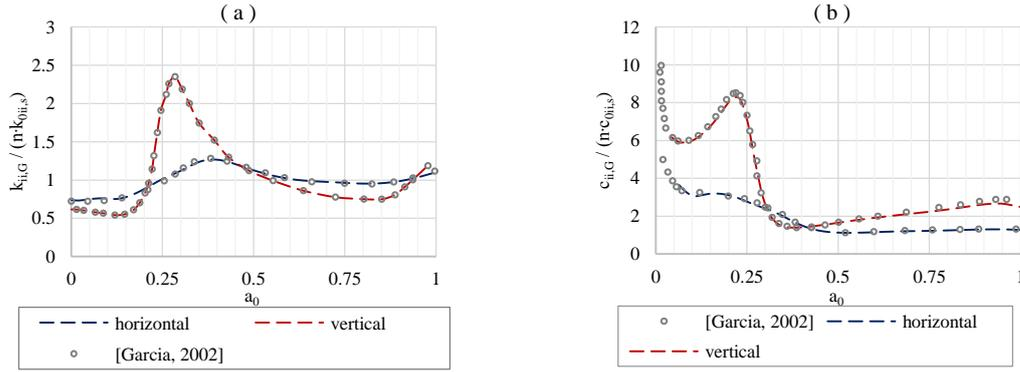
Figure 1. Dynamic impedance function in horizontal and vertical direction of a 2x2 pile group. (a) contains the real part, (b) the imaginary part.
