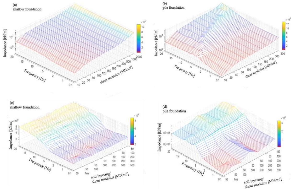
Figure 4. Horizontal impedance functions for shallow (left) or pile-grid foundations (right) on homogenous (top) and layered soil (below).
