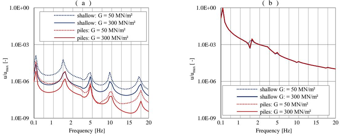
Figure 5. Normalized displacement response at the foundation top edge (left) and at the tower top (right) under a virtual load applied at the tower top node.
