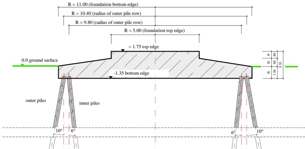
Figure 2. Geometry of the shallow and pile foundations.
