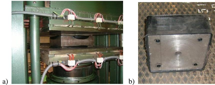
Figure 1. a) Vulcanization of the isolator b) View of the isolator
