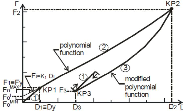
Figure 5. Polynomial analytical model of bearings made of rubber
