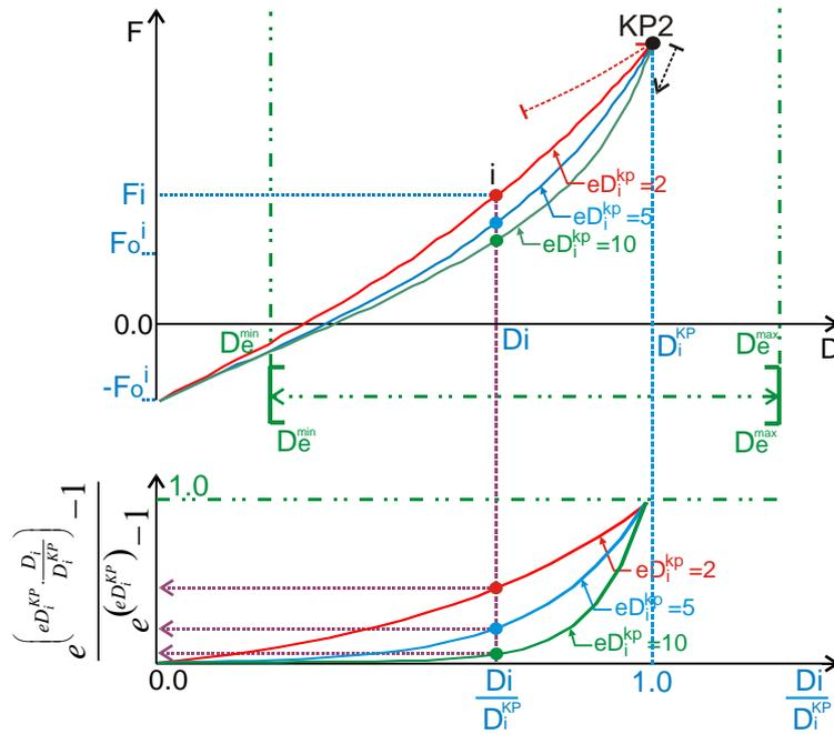
Figure 7. Dependence of the exponent on the horizontal deformation of the bearing
