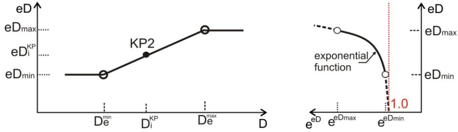
Figure 6. Dependence of the exponent on the horizontal deformation of the bearing
