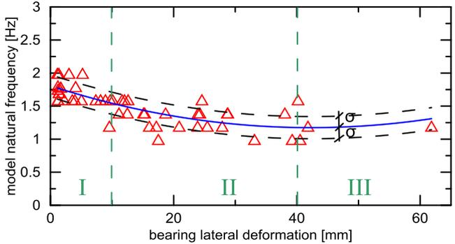
Figure 9. Shear deformation - model frequency relationship
