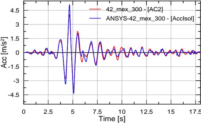
Figure 10. Comparison of time histories of acceleration at the isolation level under excitation EQ1
