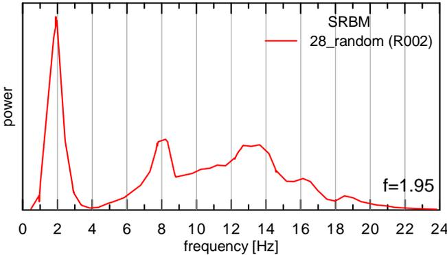
Figure 8. Frequency curve for base isolated structure
