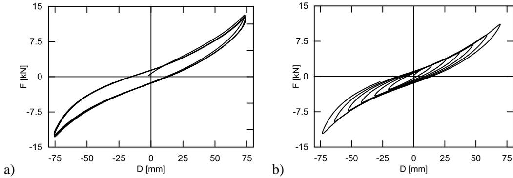
Figure 4. Relationship between horizontal displacement and horizontal force for cylindrical rubber bearings: a) constant amplitudes b) increasing amplitudes
