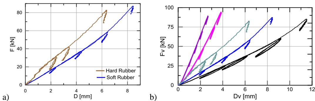
Figure 2. Relationship between vertical stiffness and vertical force 2) hard and soft compound b) different rubber compounds
