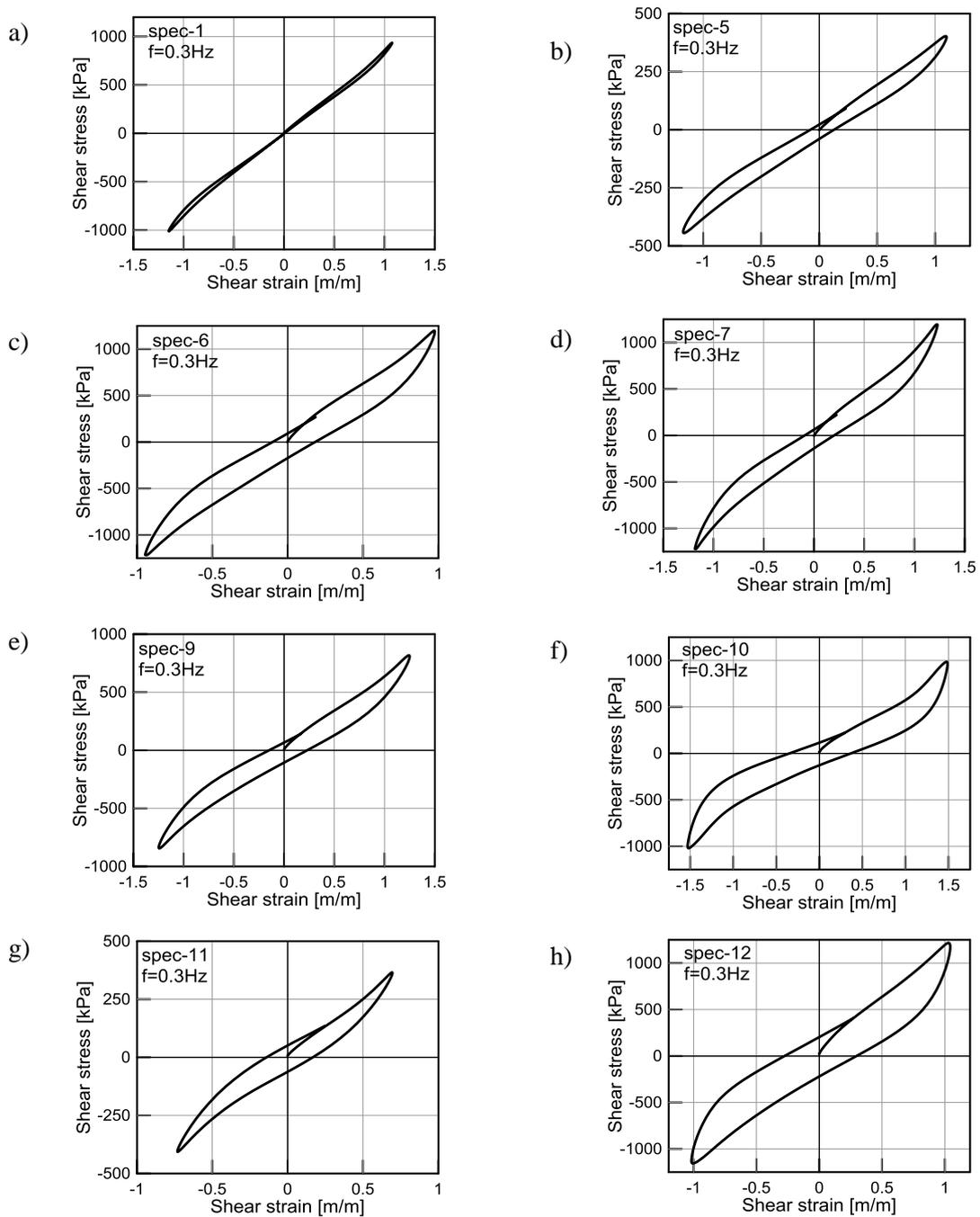
Figure 3. Comparison of horizontal behavior of bearings made of eight different rubber compounds
