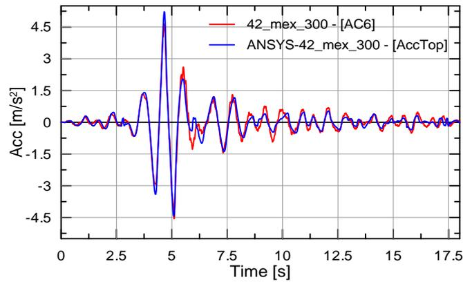
Figure 11. Comparison of time histories of acceleration at the top of the structure under excitation EQ1
