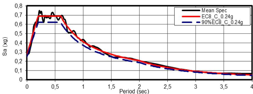
Figure 6. Average elastic spectra of scaled input motions
