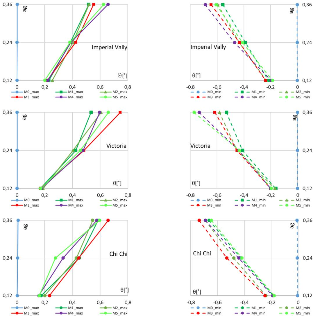
Figure 9. Maximal rotation of the  $V^{\text{th}}$  story
