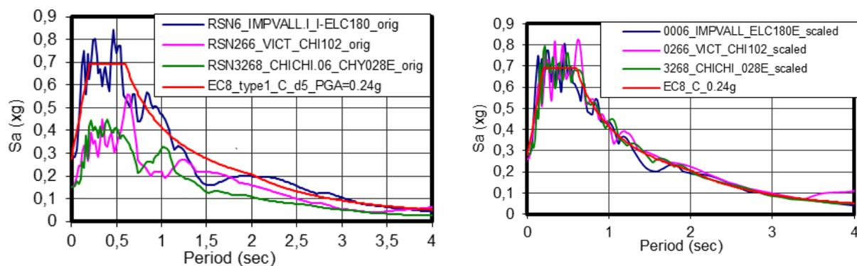
Figure 5. Elastic spectra for original and scaled input motions
