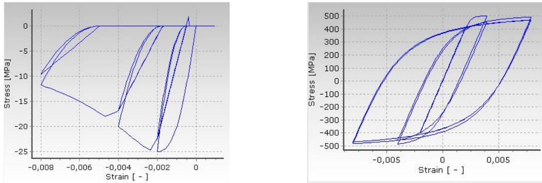
Figure 3. Mechanical characteristics for concrete and rebar
