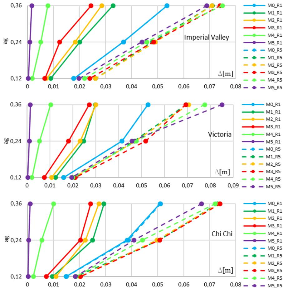
Figure 8. Maximal relative story drifts for frames R1 and R5 of the analyzed structures
