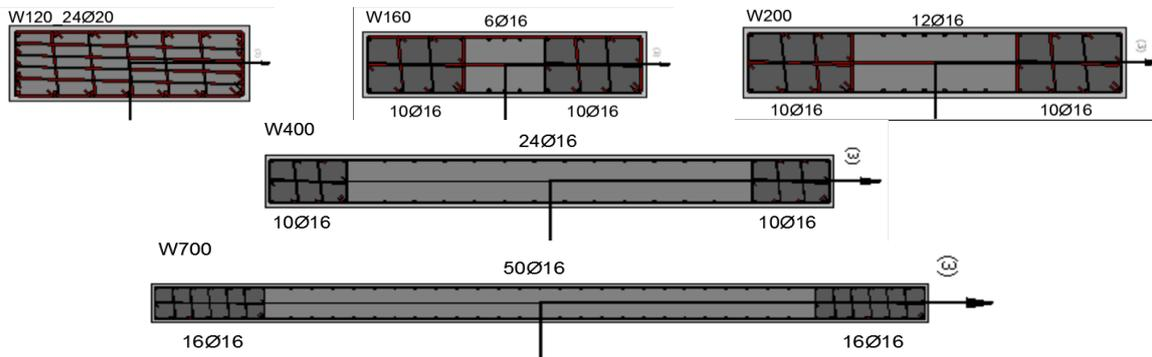
Figure 4. Reinforcement pattern in walls
