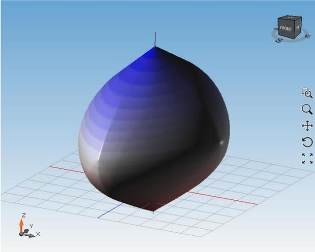
Figure 5. 3D failure surface of a rectangular section constructed with the software
