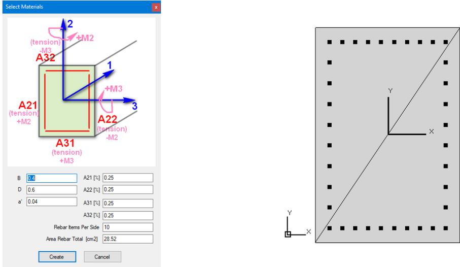
Figure 8. The analyzed cross-section data (left) and CDT mesh discretization (right)
