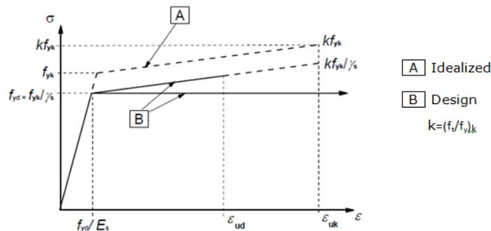
Figure 2. Idealized and design stress-strain diagrams for reinforcing steel, EN 1992-1-1 (2004)
