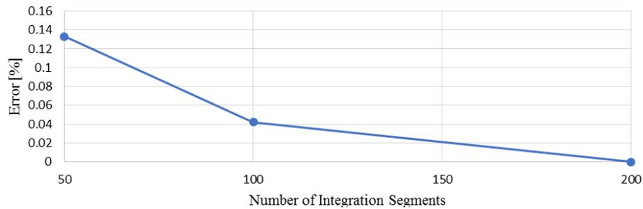
Figure 11. Dependence of error on number of integration segments for predefined section rotation of 30°
