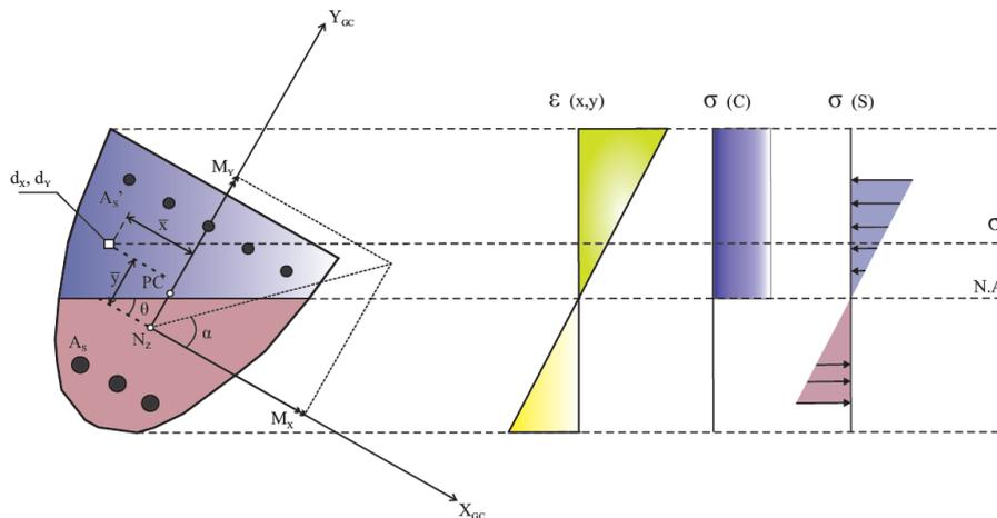
Figure 4. Stress and strain diagrams of a cross-section subjected to bending about an arbitrary axis
