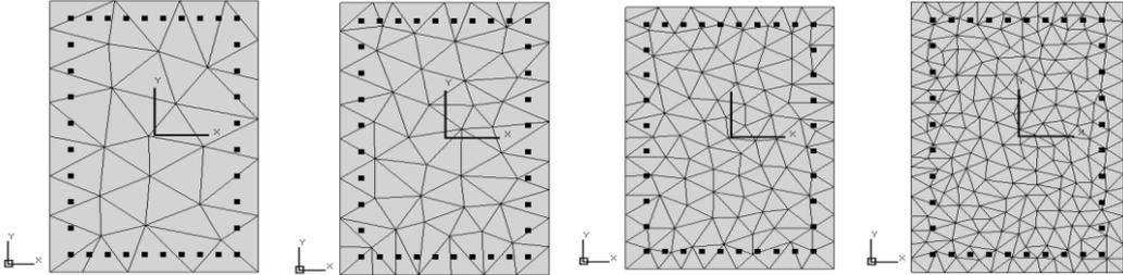
Figure 9. CCDT mesh discretization with maximum element area of 0.008, 0.004, 0.002 and 0.001 m<sup>2</sup>
