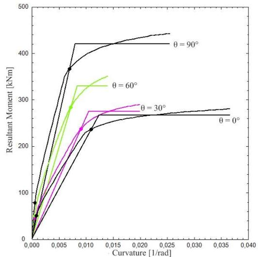
Figure 7. 3D and 2D moment-curvature representation of a rectangular section constructed with the software
