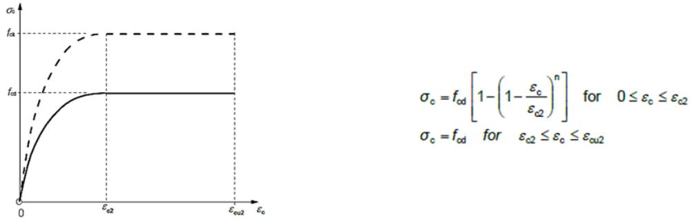
Figure 1. Parabola-rectangle stress-strain diagram for concrete, EN 1992-1-1 (2004)
