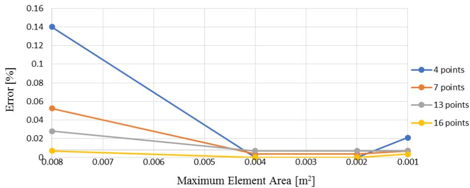
Figure 12. Dependence of error on element area for predefined section rotation of 30° (only CCDT mesh)
