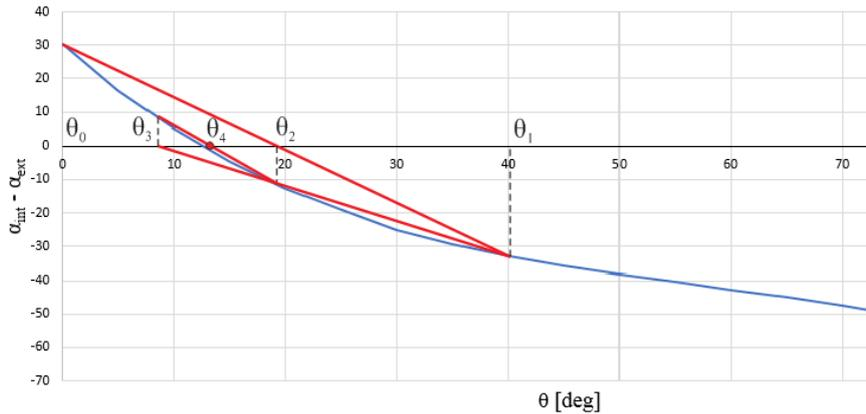
Figure 6. Secant method example for estimation of the angle of neutral axis
