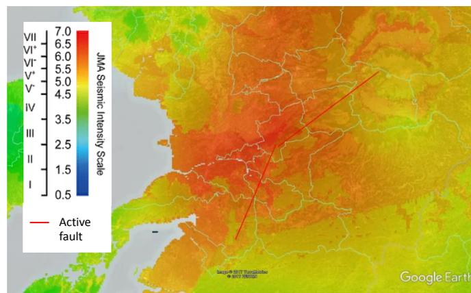
Figure 3. Strong ground-motion distribution during the Kumamoto Earthquake
