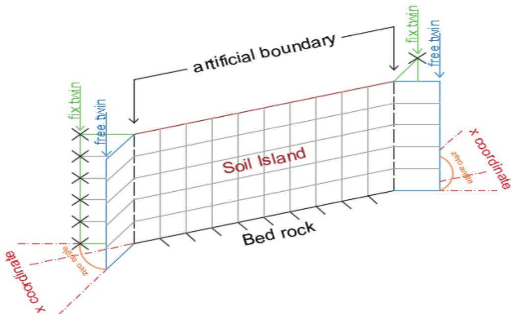
Figure 2. 2D Modeling of Main Model and Twin Boundary – Inclined View
