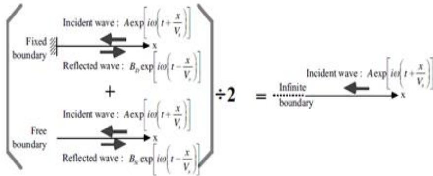
Figure 1. Incident and Reflected Waves Form Fix and Free Ends (Towhata 2008)
