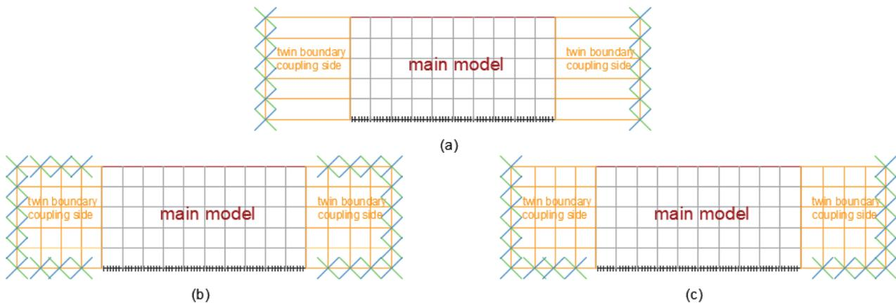
Figure 8. (a) Side Coupling; (b) Side-Bottom-Top Coupling; (c) Side-Bottom Coupling
