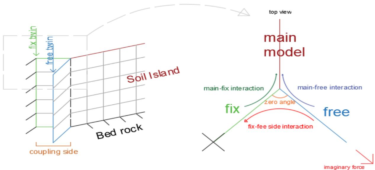
Figure 6. Available Interaction Between Coupling Side Branches and Main Model
