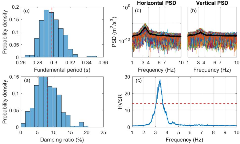
Figure 7. Results from 282 HVSR: (a) Histograms of the fundamental period and damping ratio. The red-dashed line on each figure is the mean value; (b) Ensemble average horizontal and vertical PSD (black solid line on each figure); (c) HVSR obtained from ensemble average PSD. The red-dashed line represents half the value of the maximum HVSR
