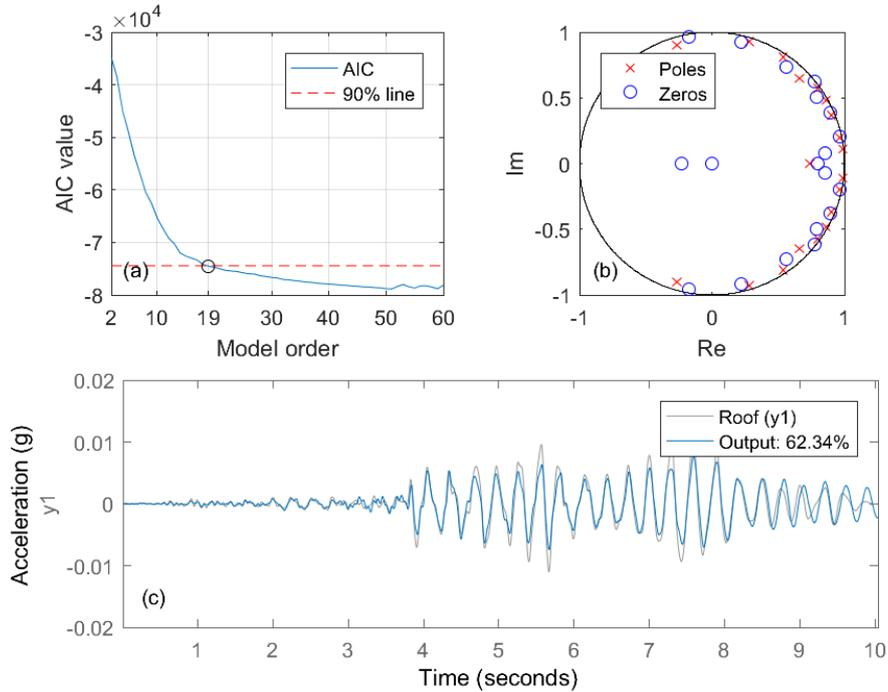
Figure 3. Selection of the optimal model order using channel-2 of aftershock no. 1: (a) AIC values for various model orders with 90% line of the minimum value, and the black circle represents 19th model order; (b) Pole-zero plot of ARX(19,19) model; (c) Output of ARX(19,19) model (blue) and the aftershock recorded at the roof (grey). The NRMSE is 62.34% in this case
