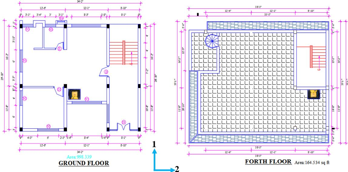
Figure 1. Ground floor and roof plan of the building being studied. The small yellow pictures indicate the locations of accelerometers installed in the building
