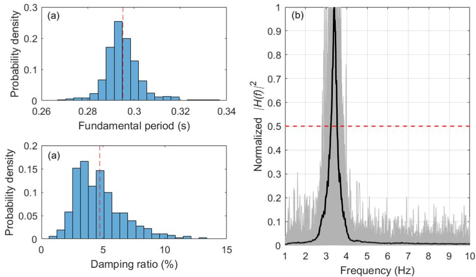
Figure 6. Results from 362 normalized  $|H(f)|^2$ : (a) Histograms of the fundamental period and damping ratio. The red-dashed line on each figure is the mean value; (b) Normalized  $|H(f)|^2$  of 362 triggered noise based on periodogram PSD estimate. The solid black line represents the normalized ensemble average
