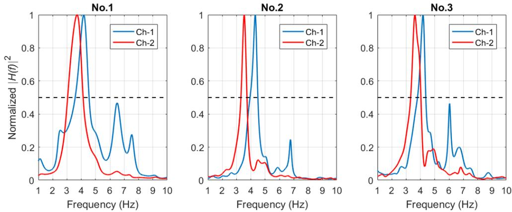
Figure 5. Normalized  $|H(f)|^2$  of frequency response function of the building computed from PSD of channel-1 and -2 of each aftershock. The black-dashed line represents the half-power line
