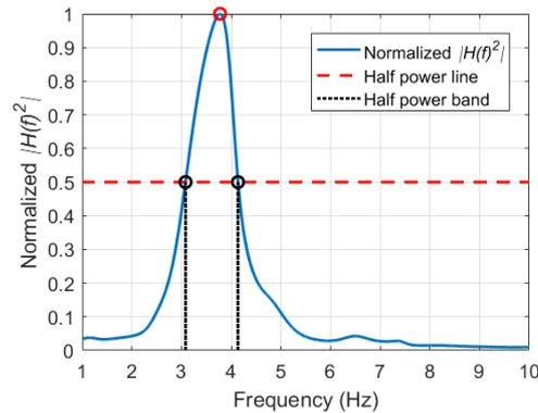
Figure 2. Example of a normalized  $|H(f)|^2$  computed from the channel-2 data of aftershock no.1
