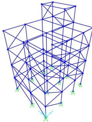
Figure 4. Finite element model of the building
