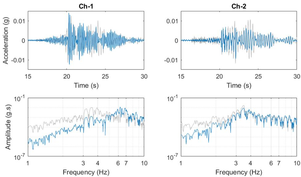
Figure 8. Acceleration and Fourier amplitude spectra at the roof in channel-1 and -2 direction for aftershock No. 1. The simulated response and recorded motion are plotted in blue and grey respectively.
