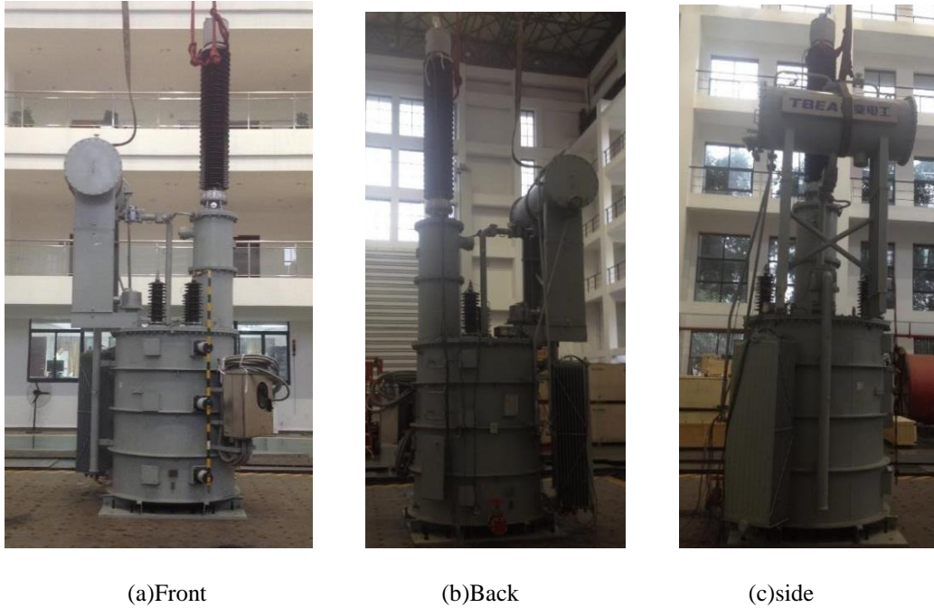
Figure 1. 220kV oil-immersed reactor for test
