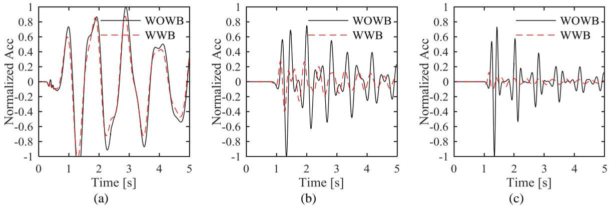
Figure. 6. Mean horizontal acceleration at soil surface under Ricker wavelet with the predominant frequency of a) 0.92 Hz b) 2.32 Hz c) 3.72 Hz
