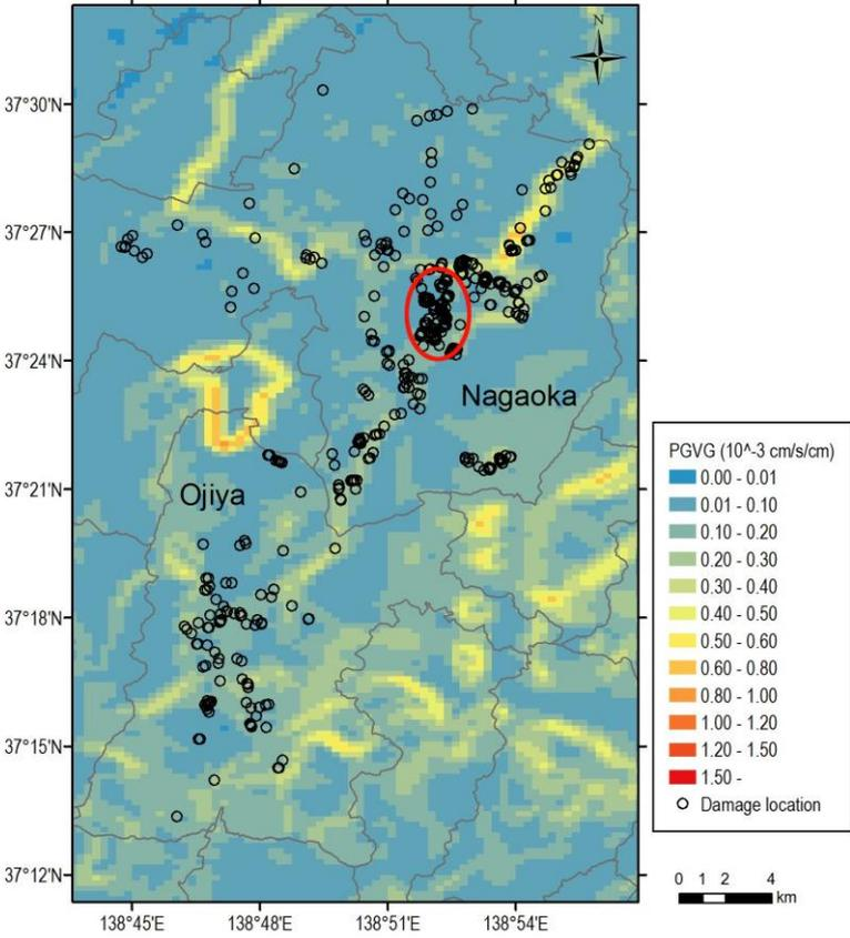
Figure 3. Simulated PGV gradient distribution and locations of WSP damage points. (Chuetsu earthquake) The region enclosed by a red ellipse, which is a landslide-affected area.
