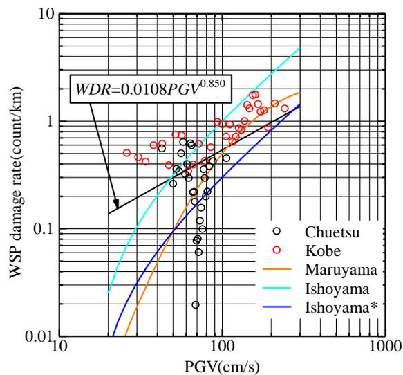
Figure 6. Relationship between the WDR and PGV values. (Kobe and Chuetsu earthquakes)
