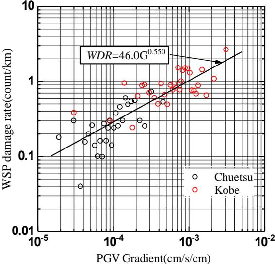
Figure 8. Relationship between the WDR and the simulated PGV gradients. (Chuetsu and Kobe earthquakes)
