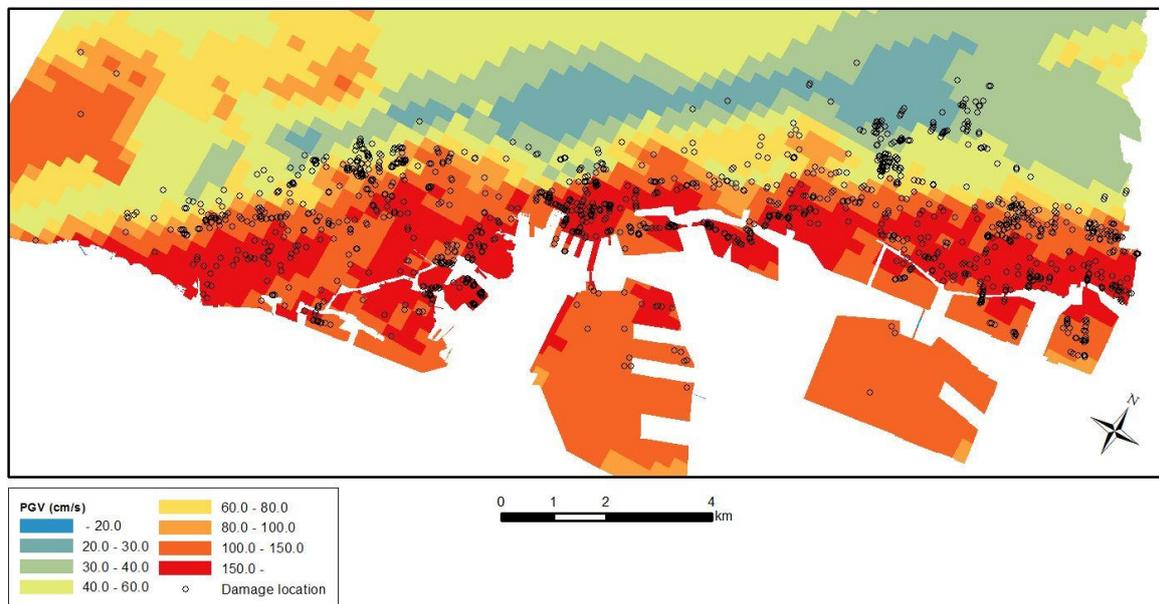
Figure 5. PGV distribution and locations of WSP damage points in Kobe city. (Kobe earthquake)
