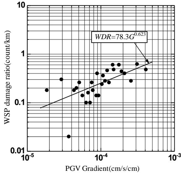
Figure 4. Relationship between the WDR and PGV gradient values. (Chuetsu earthquake)
