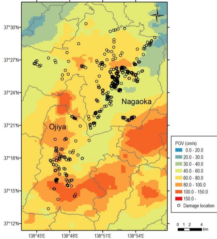
Figure 1. Simulated PGV distribution and locations of WSP damage points. (Chuetsu earthquake)
