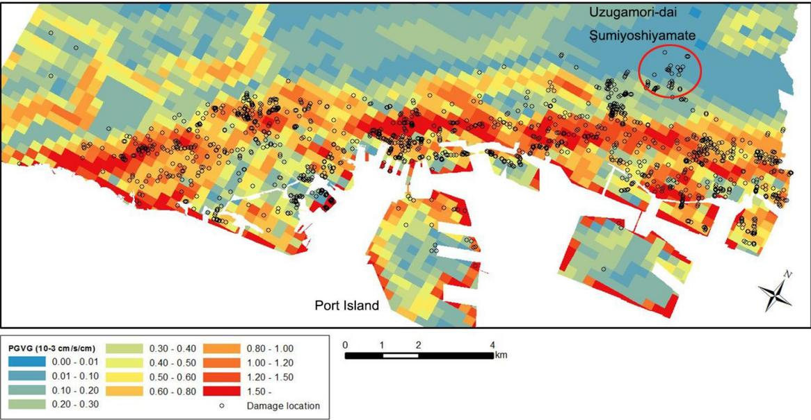
Figure 7. PGV gradient distribution and locations of WSP damage points. (Kobe earthquake)
