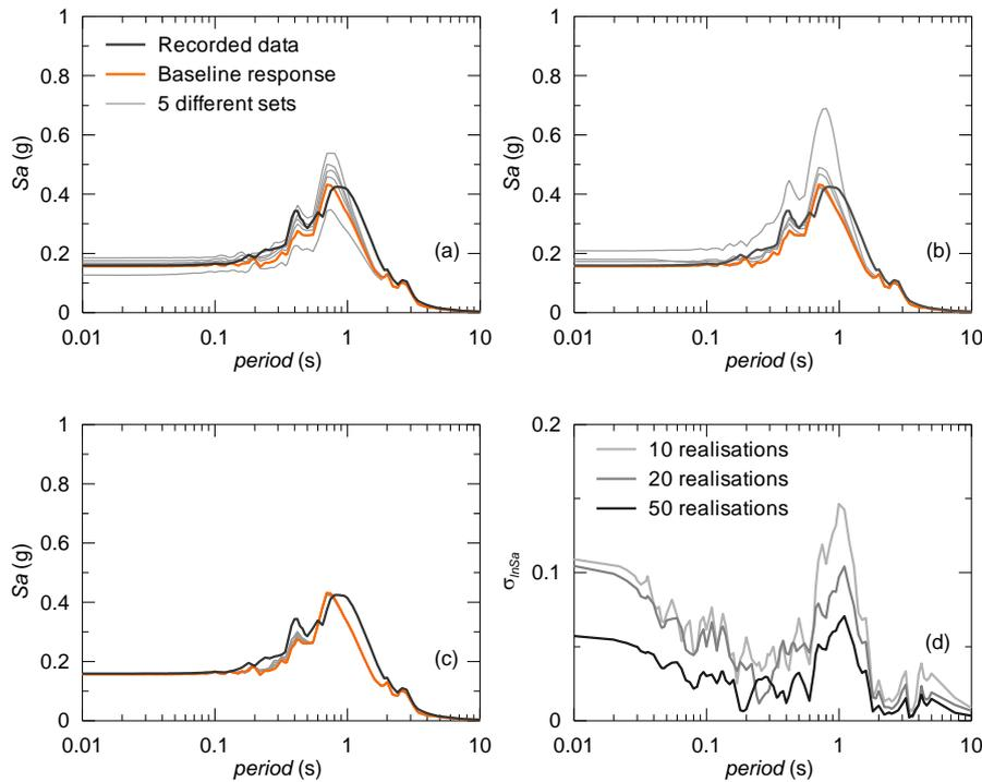
Figure 4. Median surface response for suites of (a) 10, (b) 20, (c) 50 realizations of nonlinear curves and (d) standard deviation of the surface response spectra
