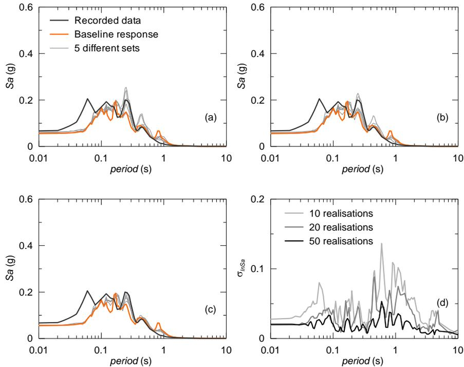
Figure 6. Median surface response for suites of (a) 10, (b) 20, (c) 50 realizations of  $V_s$  profile and (d) standard deviation of the surface response spectra
