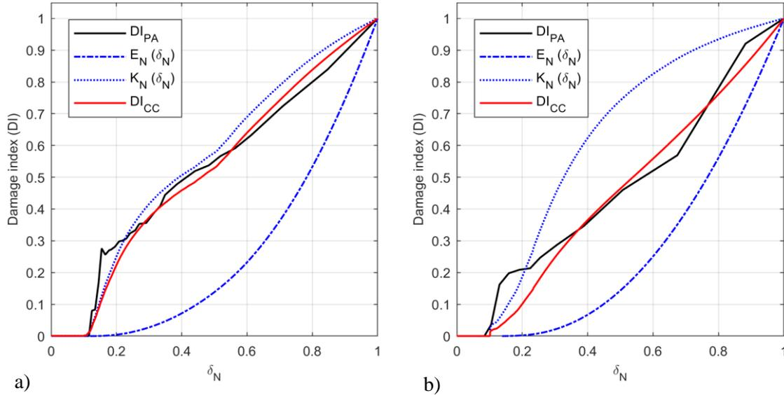
Figure 6.  $DI_{CC}$  defined from capacity curves for: a) RCM structure and b) DRC structure.
