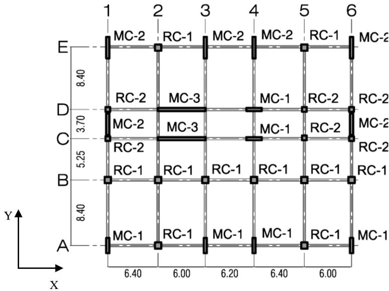
Figure 2. Plan view of the vertical structural elements distribution for the DRC structure.
