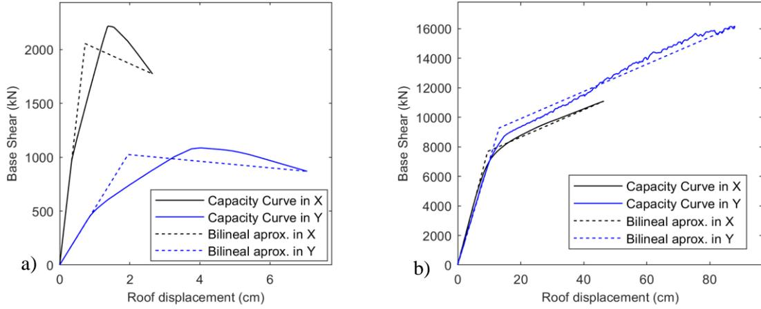
Figure 4. Capacity curves from a Pushover analysis for: a) RCM structure and b) DRC structure.
