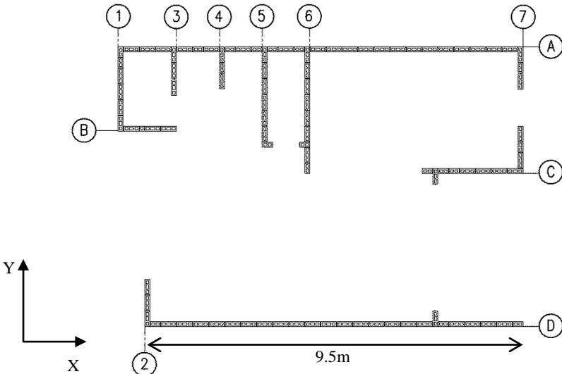
Figure 1. Walls distribution on the first floor of the RCM structure.
