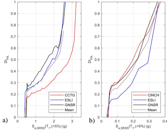
Figure 5. Variation of the  $DI_{PA}$  as a result of the IDA for: a) RCM structure and b) DRC structure.
