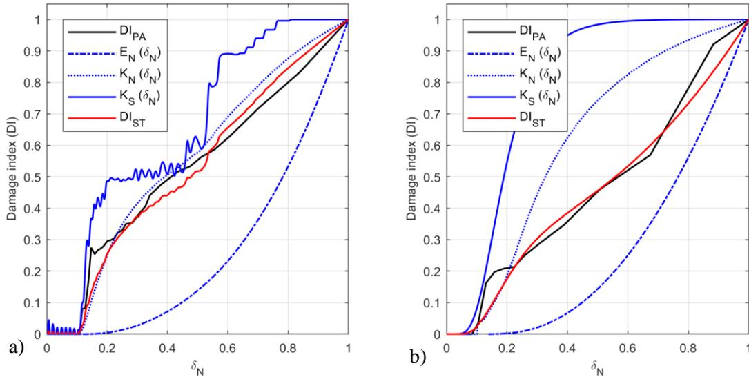
Figure 7.  $DI_{ST}$  defined from capacity curves for: a) RCM structure and b) DRC structure.
