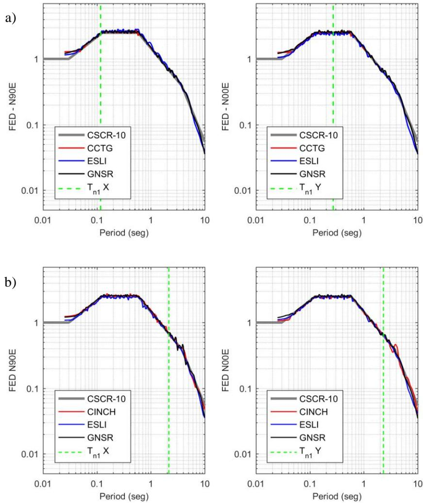
Figure 3. Response spectra of spectrally matched records in the two main direction of analysis for: a) RCM structure and b) DRC structure.
