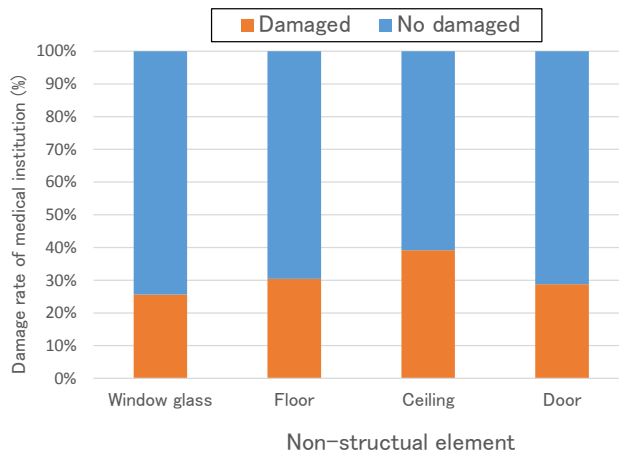
Figure 7. Damage rate of non-structural element
