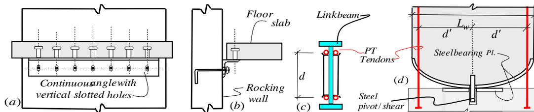
Figure 3. (a) and (b) Wall-slab shear connection, (c) LB section, (d) Rocking wall base and cables
