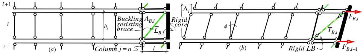
Figure 5. (a) Subframe  $i$  and BRB before rotation, (b) Subframe  $i$  and BRB after rotation
