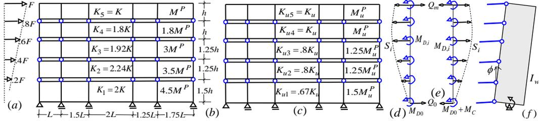
Figure 7. (a) Loading, (b) MFUR sub-frame stiffnesses and plastic moments (c) MFUS sub-frame stiffnesses and beam plastic moments (d) Interactive forces on MF (e) Interactive forces on RRW
