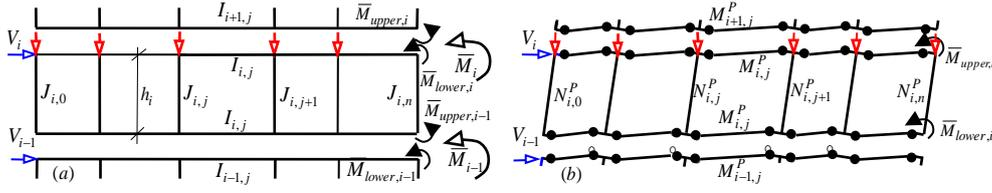
Figure 4. (a) Subframe under racking shear and LB moments, (b) Subframe plastic failure mechanism.
