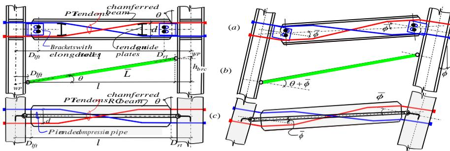
Figure 2. (a) Chamfered steel LB, (b) BRB (c) Chamfered reinforced concrete LB.
