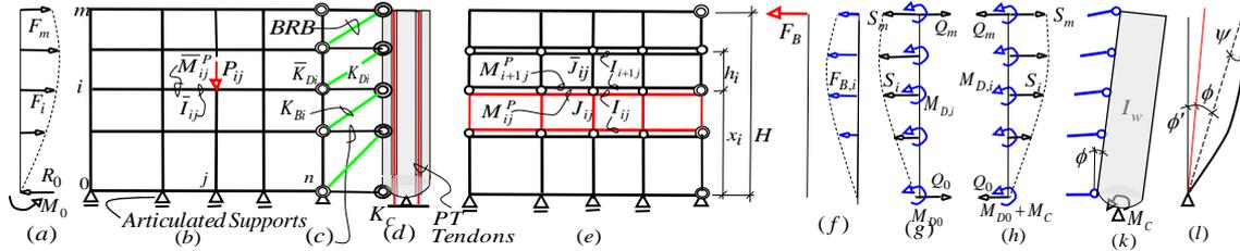
Figure 1. (b) GBRMF, (c) LBs, (d) RRW, (e) Equivalent sub-frames, (f) BRB shear distribution, (g) LB forces acting on MF (h) LB forces acting on RRW, (k) RRC base moment, (l) RRW displacements
