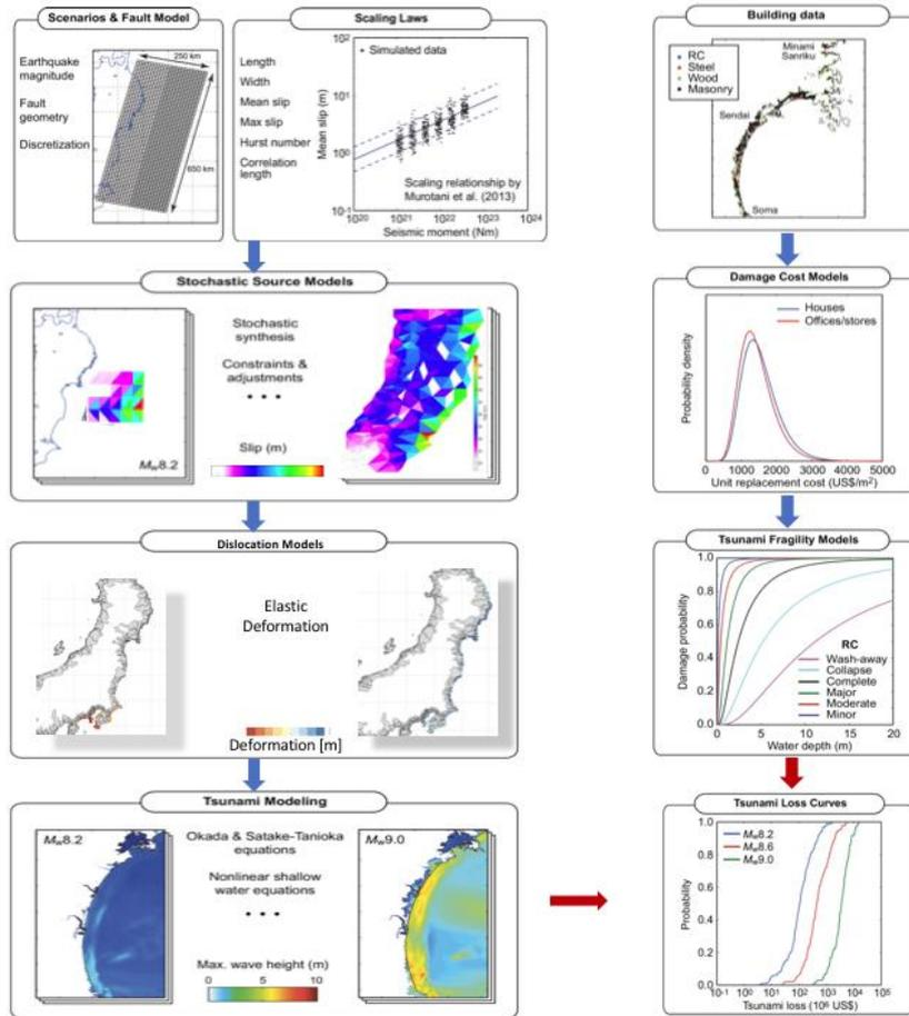
Figure 1. Schematic procedure for a Probabilistic Tsunami Hazard Assessment (PTHA). Figure adapted and modified from (Goda and Abilova, 2016).
