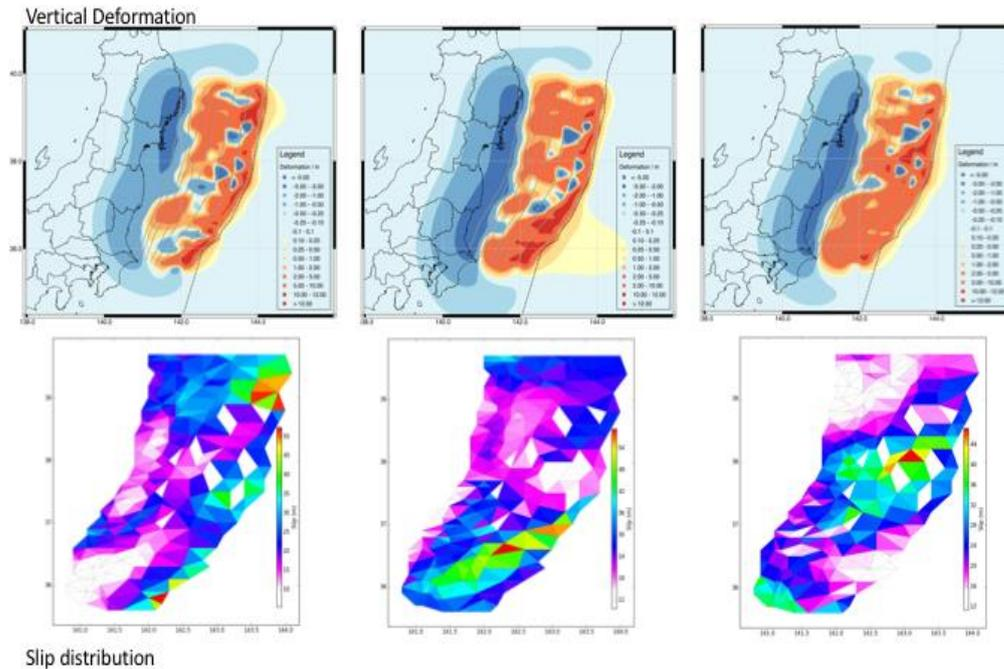
Figure 4. (Bottom row) Scenario slip distributions for the M9-type Tohoku sources. (Top row) Vertical elastic deformation pattern corresponding to the slip distributions below.
