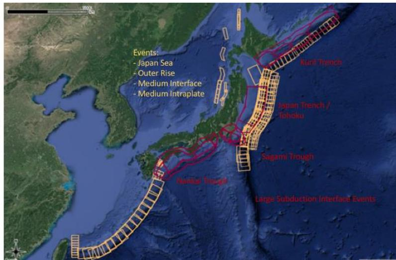
Figure 2. Location of tsunamogenic earthquake sources for the RMS Japan PTHA model. Colours differentiate large subduction interface events (red) and other offshore events that are assumed to generate tsunamis (yellow).
