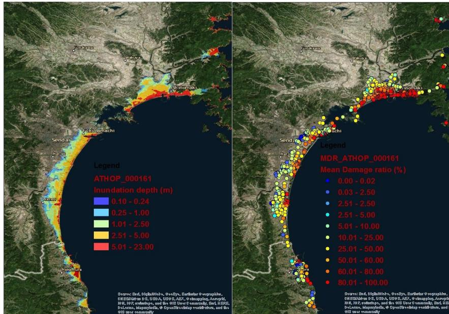
Figure 10. Left: Inundation map of one of the stochastic tsunami event. Right: Corresponding Mean Damage Ratios (MDR)
